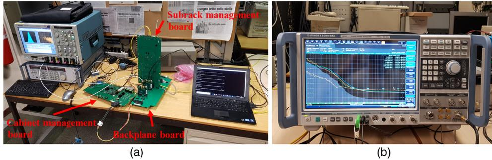
**Fig. 13** Measurement setup of the 10-MHz clock signal distributed through the chain composed of cabinet management board, SMB and backplane board: (a) the circuit under test is in the middle, its output is connected to the oscilloscope (left) and a PC (right) controls the board registers and (b) R&S FSWP50 phase noise analyzer.
