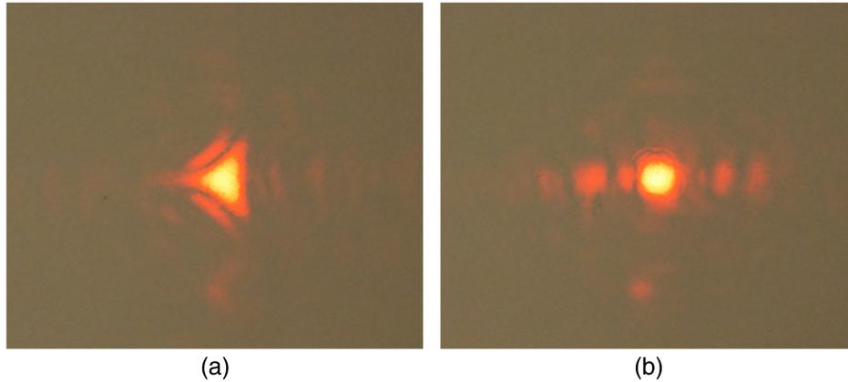
**Fig. 5** A HeNe laser signal is emitted from a fiber optic at the focal point of each OAP; the images above show the resulting collimated beam refocused by (a) an off-the-shelf OAP mirror produced by Edmund (Stock #35-491) and (b) a custom fabricated OAP by Nu-Tek. The former produces a strong coma, whereas the latter produces a smaller overall spot and does not display significant low order aberration. Both images are shown at the same physical scale.
