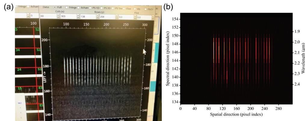
**Fig. 11** ABCD chip observations appear on the detector as a series of 24 parallel lines, measuring four phases of the visibility contrast at each wavelength channel. (a) Several outputs show regular light and dark bands along the spectral direction, indicating unoptimized optical path delay at the time this photo was taken. (b) The optical path delay is corrected and for each baseline, the ABCD outputs show varying flux intensity indicative of measured fringe contrast.
