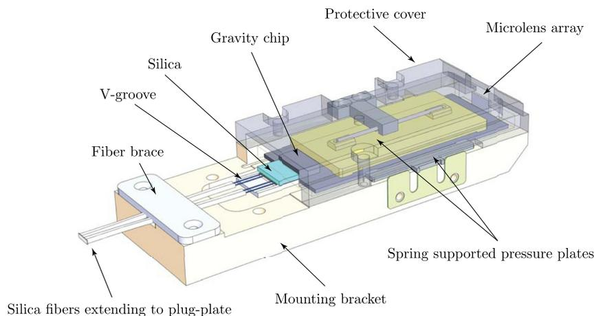
**Fig. 12** Schematic of the ABCD combiner assembly prepared at IPAG. Note that the cover protecting the GRAVITY chip from incidental damage is made transparent in this diagram for illustrative purposes only.
