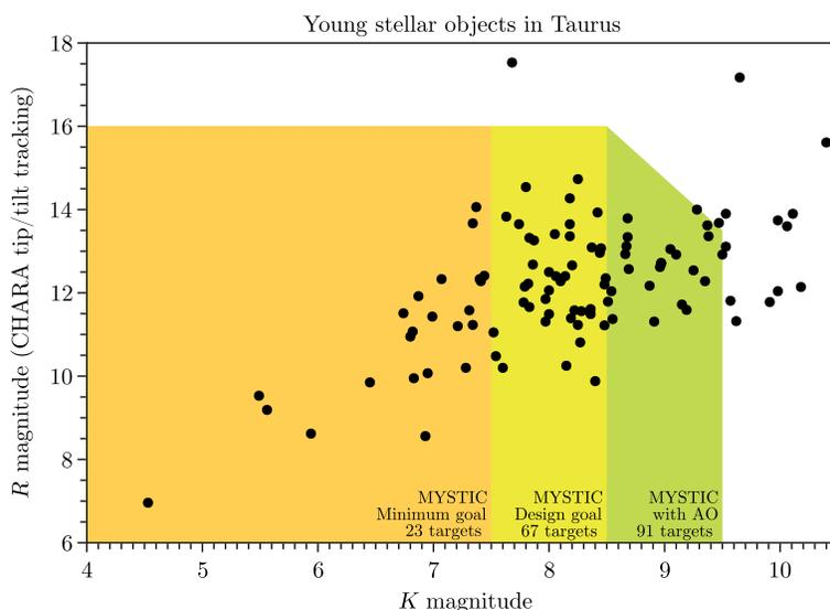
**Fig. 2** Required instrumental sensitivity to observe YSO targets in the Taurus-Auriga molecular cloud region,<sup>9</sup> which drove the design specification of MYSTIC. Currently, MYSTIC as-built meets the minimum specification (orange region). Planned future upgrades (see Sec. 10) will deliver an increase of at least 1 magnitude in sensitivity (yellow region) which more than doubles the number of available objects for study.
