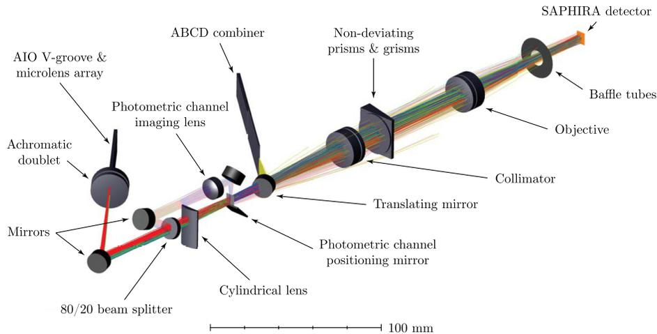
**Fig. 9** Annotated layout of the cold optic system, with beam trains for both combiners overlaid. To the left of the translating mirror are the AIO mode optics. This mirror slides out of the beam train for AIO mode observations or into the beam train for ABCD mode observations.
