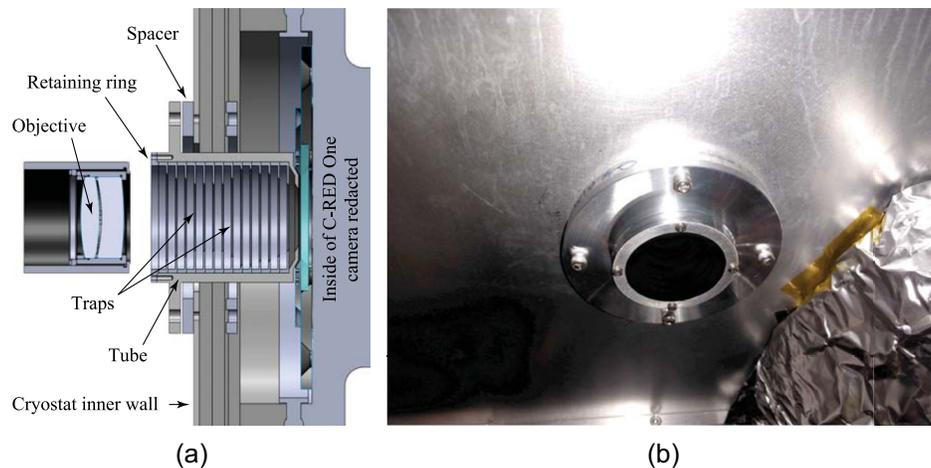
**Fig. 7** (a) Position and schematic cut view of the baffle tube assembly and (b) an image of the baffle tube mounted on the inner wall of the MYSTIC cryostat. The baffle tube consists of a series of varying inner-diameter traps coated in Singularity Black paint, which absorb stray thermal background light.
