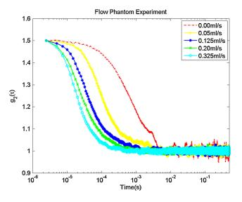
Fig. 6 Autocorrelation curves of the phantom with varied speed of flow (0 ml/s, 0.05 ml/s, 0.125 ml/s, 0.2 ml/s, and 0.325 ml/s) as a function of delay time,  $\tau$ .
