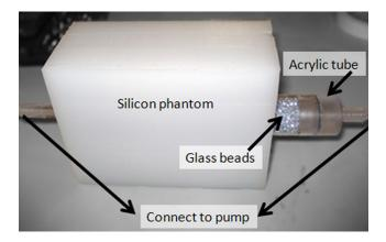
**Fig. 4** The in-house silicon flow phantom, in which an acrylic cylindrical tube was embedded to mimic the blood vessel. The tube was filled up with glass beads with a diameter of 3 mm in order to make random flow directions.
