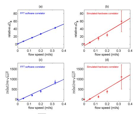
**Fig. 8** Linearity test of relative BFI (either  $\alpha D_B$  or  $\sqrt{\alpha \langle V^2 \rangle}$ ) versus flow speed. (a) and (c) are obtained using a software autocorrelator (shown in blue), while (b) and (d) are obtained using a hardware autocorrelator (shown in red). All rBFIs are normalized to the BFI value at zero flow.
