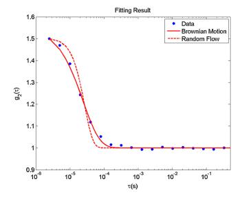
**Fig. 7** Comparison between Brownian motion and the random flow model. The autocorrelation function was calculated from the flow phantom data with a speed of 0.325 ml/s. The entire autocorrelation data was sampled and shown as dots.
