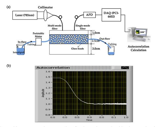
Fig. 5 (a) Schematic of the DCS experimental setup using in-house flow phantom. (b) Screen shot of the LabVIEW interface of the FFT-based autocorrelation calculation.
