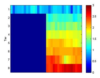
**Fig. 2** A snapshot of the registers of simulated hardware correlator. Color represents the logarithm of the photon count in each register. Ignore the blue portion on the left where there are no registers.
