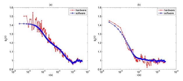
**Fig. 3** Comparison between hardware and software autocorrelation calculations. (a) Autocorrelation calculated from a typical flow phantom data. (b) Autocorrelation calculated from a simulated data. Hardware-simulating algorithm (red squares) was implemented under the assumption of a 10-tier register, averaged over 500 different autocorrelations. The sampling rate was 400 kHz.
