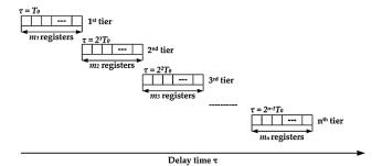
**Fig. 1** The diagram of hardware autocorrelator inner structure, with several tiers of registers where the delay times are the power of two times of initial delay time  $T_0$ .
