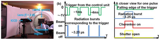
**Fig. 1** (a) Relative positions of the linear accelerator (LINAC) gantry, treatment region, and the time-domain gated system. The intensified charge coupled device (ICCD) was synchronized to radiation bursts from the LINAC and Cherenkovscopy were taken from the beam incident on the treatment regions. (b) Timeline about the temporal gating.
