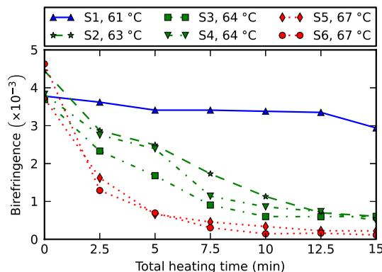
**Fig. 2** The mean birefringence of porcine tendon samples (S1 to S6) after thermal stress. Samples were immersed in heated Krebs solution at the indicated temperatures;  $61^\circ\text{C}$  (blue),  $63^\circ\text{C}$  to  $64^\circ\text{C}$  (green), and  $67^\circ\text{C}$  (red). Total heating time refers to the duration of the applied thermal stress.
