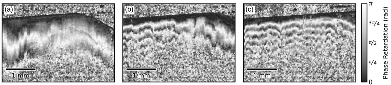
**Fig. 3** Phase retardation B-scans of a porcine tendon sample after partial immersion into 69°C Krebs solution for 5 min. (a) From a section of the sample which was immersed into solution. (b) From the boundary between the immersed (right) and nonimmersed (left) regions. (c) From the nonimmersed region.
