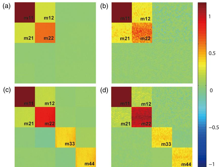
**Fig. 3** Experimental and simulation results of forward scattering Mueller matrix. (a) and (b) are experimental and simulated results of birefringent cylinders (well-aligned silk fiber). (c) and (d) are experimental and simulated results of nonbirefringent cylinders (well-aligned glass fiber).
