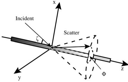
**Fig. 1** Schema of the single light scattering by infinite cylinder.
