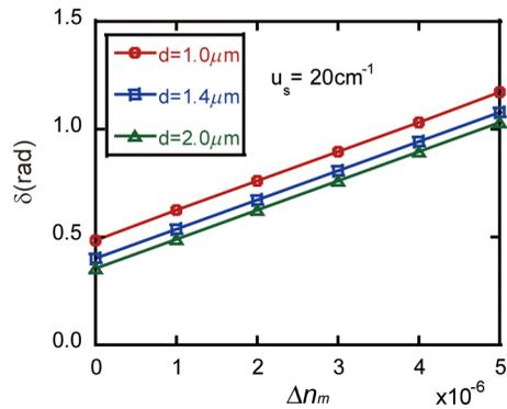
**Fig. 6** Change in the birefringence of the medium surrounding the nonbirefringent cylinder. The diameters of the cylinder were 1.0, 1.4, and 2.0  $\mu\text{m}$ , and the scatter coefficient is  $\mu_s = 20 \text{ cm}^{-1}$ ; the birefringence of the ambient medium  $\Delta n_m$  varies from 0 to  $5 \times 10^{-6}$ .
