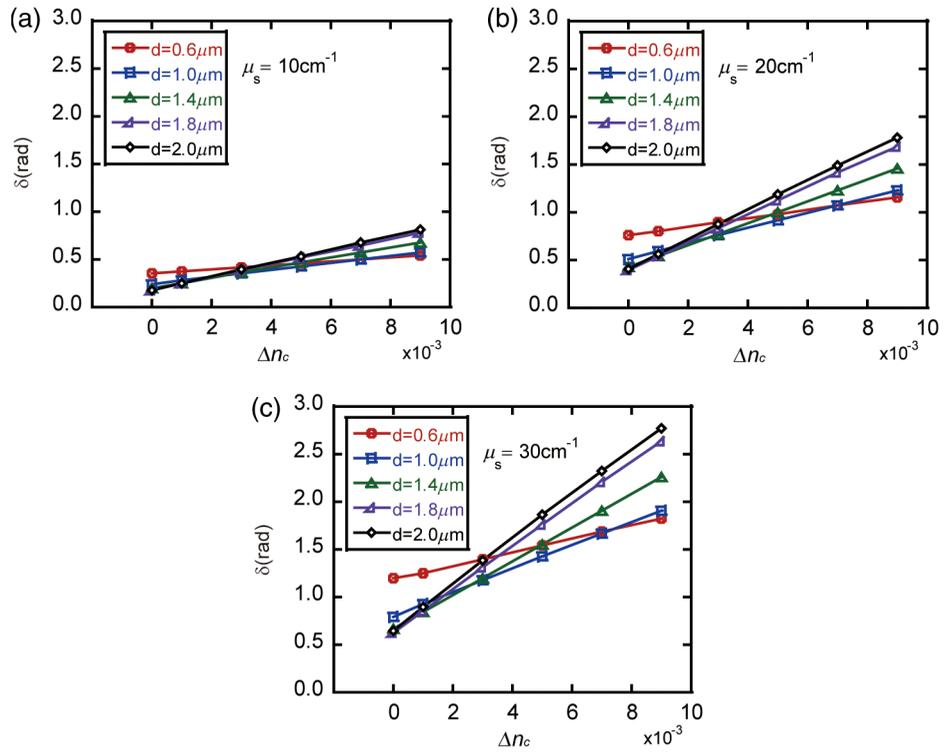
**Fig. 4** The relationship between the birefringence of the cylinders and the retardance  $\delta$ . Different curves represent different diameters of birefringent cylinders, (a)–(c) represent different scattering coefficients of the sample.
