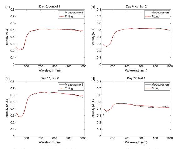
Fig. 2 Examples of the fitting to the single-fiber spectroscopy measurements. (a) Day 0, control 1; (b) day 0, control 2; (c) day 12, test 6; and (d) day 77, test 1.
