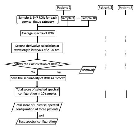
Fig. 7 The calculation process of screening filter.
