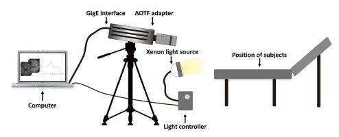
Fig. 1 Schematic view of the integrated hyperspectral imaging system for high-grade (HG) lesion detection.
