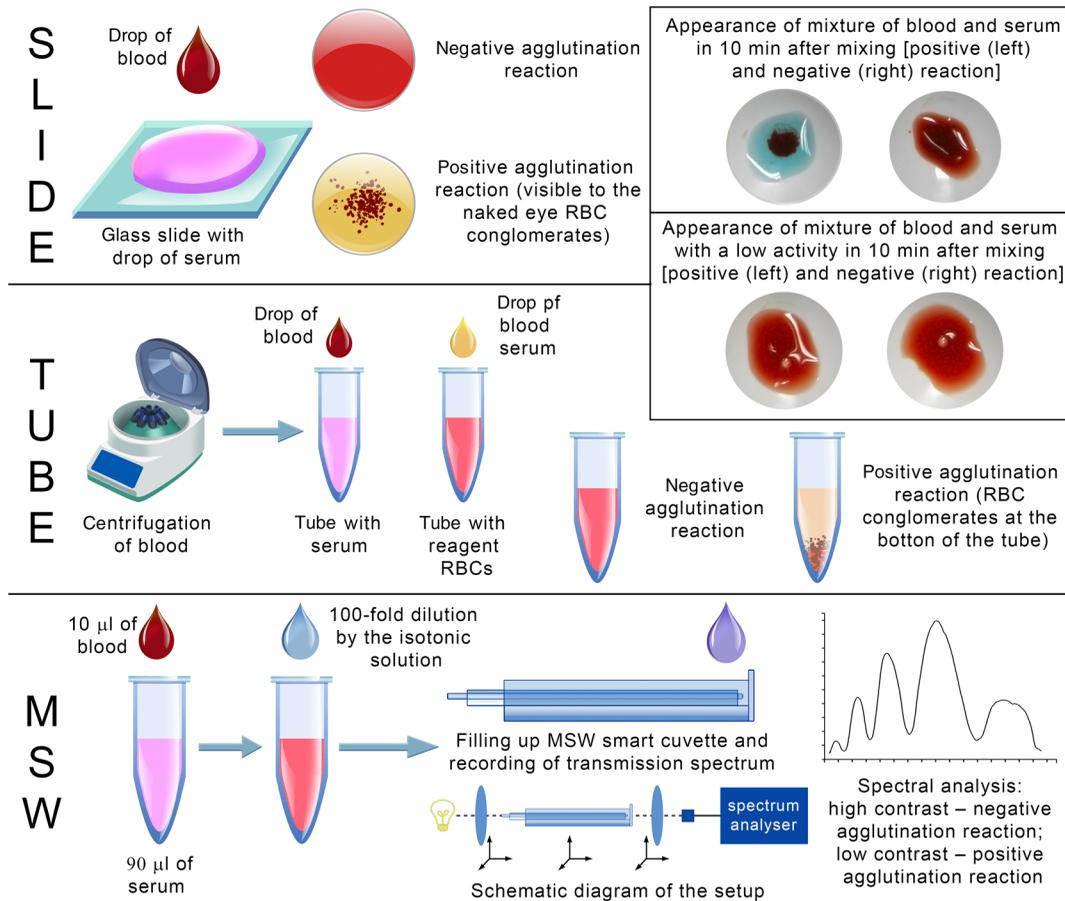
**Fig. 2** Slide, tube, and MSW methods for blood typing. Top right: photographs of mixtures of whole blood and standard sera with normal and low activities.
