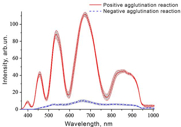
**Fig. 3** Transmission spectra of identical 60-mm-long MSW smart cuvettes filled by the products of positive (+) and negative (–) reactions of blood. Spectra were averaged over nine independent measurements with hatched areas showing the absolute errors of each measurement.
