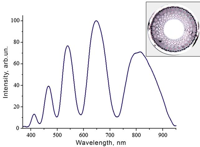
**Fig. 1** The transmission spectrum of a microstructured waveguide (MSW) (hollow core diameter is 150  $\mu\text{m}$ ). The top right insertion is the electronic micrograph of the MSW cross section.
