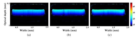
**Fig. 7** Optical coherence tomography (OCT) images of capillary cross section with nanoparticle (NP) suspensions of (a) NSts, (b) NCs-7, and (c) NCs-52. Brighter color indicates higher scattering at  $\lambda = 930$  nm. Inner capillary thickness is 200  $\mu$ m. Adapted from Ref. 40.
