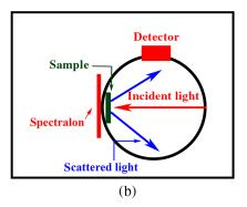
Fig. 2 Schemes for measuring (a) collimated transmission and (b) absorption.
