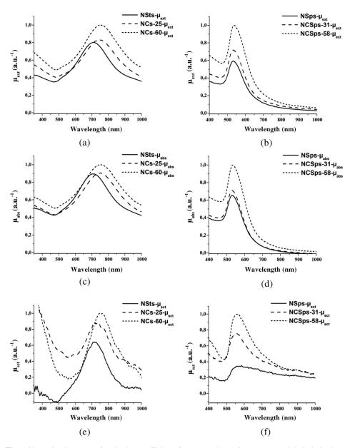
**Fig. 5** Normalized spectra of extinction coefficients for suspensions of nanostars and their derivatives; (b) nanospheres and their derivatives; (c) spectra of absorption coefficients of nanostars and their derivatives; (d) nanospheres and their derivatives; (e) spectra of scattering coefficients of nanostars and their derivatives; and (f) nanospheres and their derivatives.
