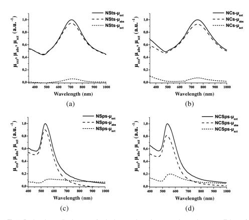
Fig. 3 Retrieved normalized spectra of extinction  $\mu_{\rm ext}$ , absorption  $\mu_{\rm abs}$ , and scattering  $\mu_{\rm sct}$  coefficients of (a) NSts, (b) NCs, (c) bare nanosphere suspensions, and (d) silica-coated (NCSps) suspensions.
