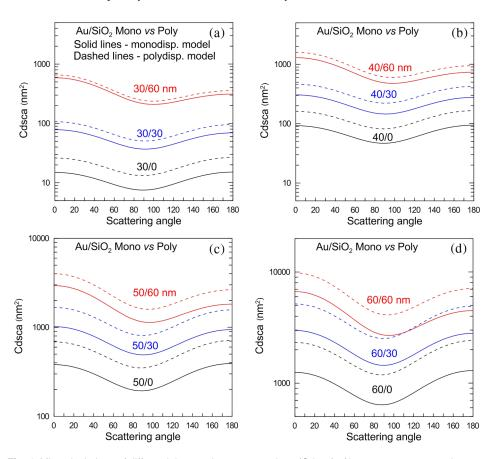
**Fig. 4** Mie calculations of differential scattering cross sections (Cdsca) of bare 30-, 40-, 50-, and 60-nm gold NPs and silica-coated NPs with a 30-nm or 60-nm silica shell. The calculations were done for both monodisperse (solid lines) and polydisperse (dashed lines) models. Standard Gaussian distribution with the normalized standard deviation = 0.3 was used for polydisperse model.
