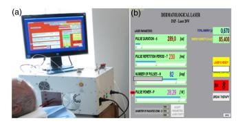
Fig. 1 Experimental setup: (a) dermatological laser and (b) control panel of the laser.
