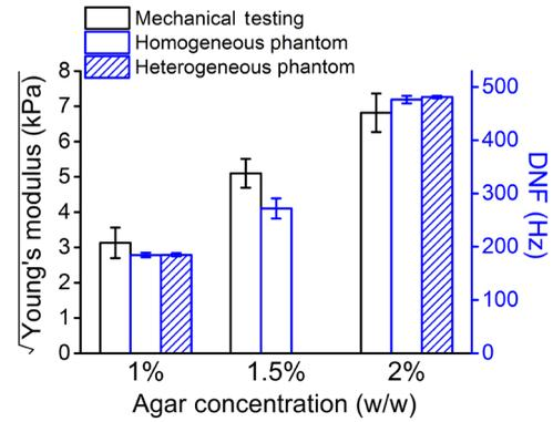
**Fig. 4** Comparison of the square root of Young's modulus as measured by uniaxial mechanical testing ( $n = 4$  samples for each concentration) to the DNF of the same homogeneous phantoms ( $n = 9$  OCE measurement positions for each concentration) and the corresponding heterogeneous phantom components ( $n = 24$  and  $57$  for 1% and 2% components, respectively). Error bars are the 95% confidence intervals of the means.
