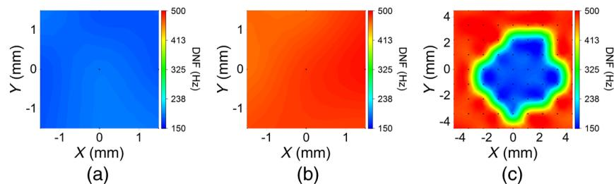
**Fig. 3** Damped natural frequency (DNF) maps in the agar phantoms where the black dots represent the OCE measurement positions, and the DNF scale is the same for direct comparison. DNF maps of the: (a) homogeneous 1%, (b) homogeneous 2%, and (c) heterogeneous phantoms.
