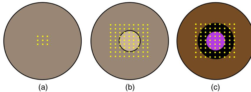
**Fig. 1** OCE measurements for the phantoms and corneas where the yellow dots represent measurement positions. 2-D grid of OCE measurements on the: (a) homogeneous phantoms, (b) heterogeneous phantoms where the lighter central region represents the 1% agar and the darker outer region represents the 2% agar, and (c) corneas where the purple region represents the masked area during the partial CXL treatment. Figures are not to scale.
