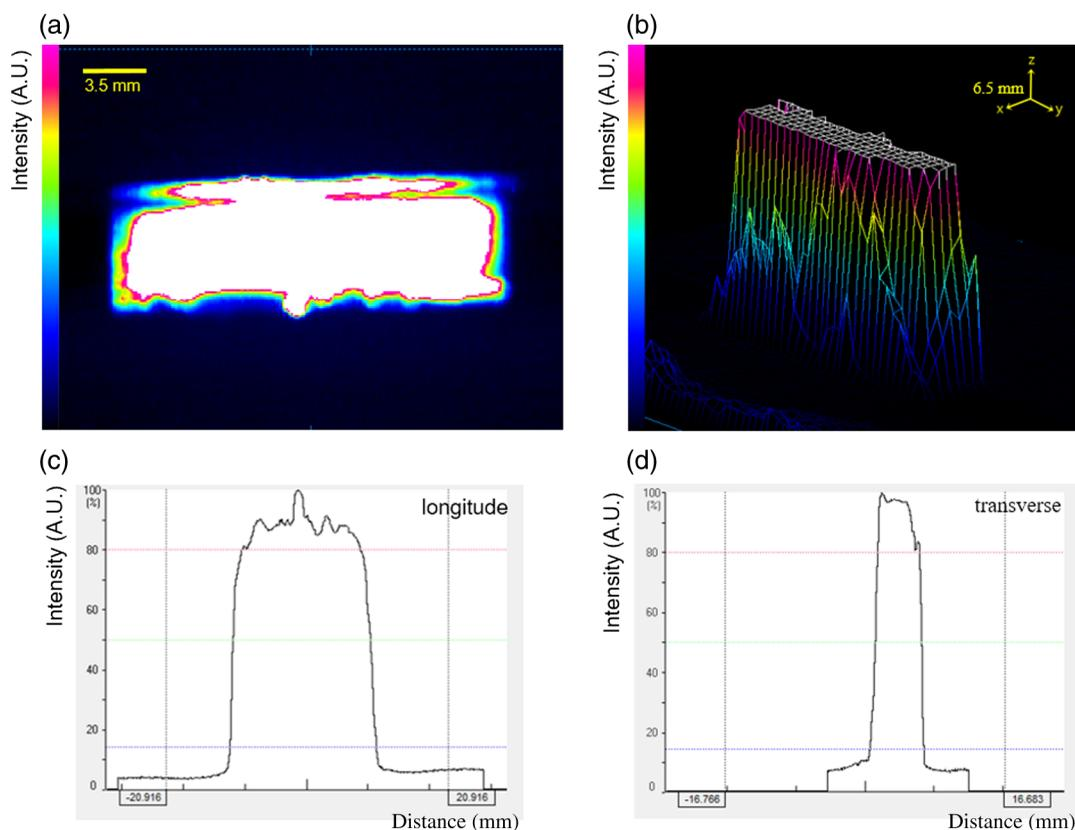
**Fig. 3** Characteristics of the proposed probe using a beam profiler. (a) Two-dimensional and (b) 3-D plots of line-shaped beam intensity showing the performance of the PAI probe; (c) and (d) longitude and transverse profiles of the beam intensity distribution.
