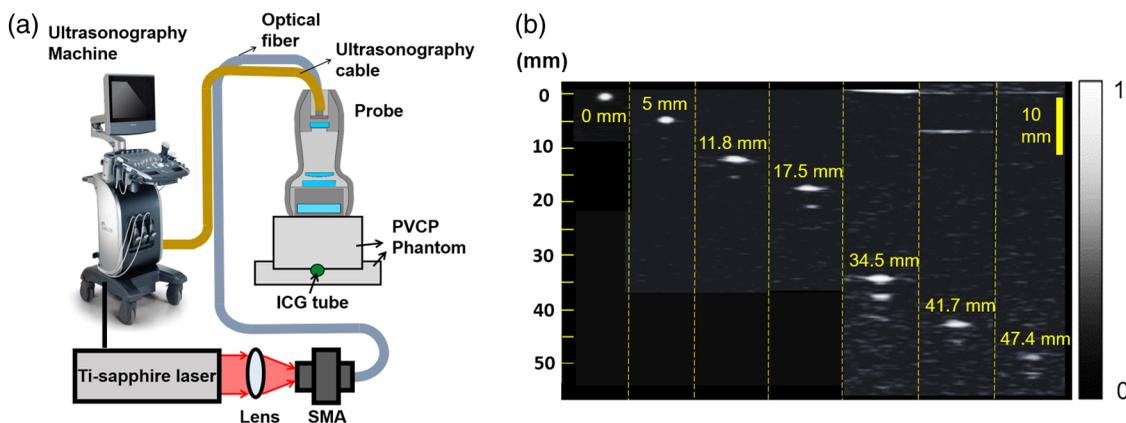
**Fig. 4** (a) Schematic of the proposed system to acquire PAI that can image immediately below the window of the PAI probe and (b) a merged image of each ICG image from the PAI system at various depths in the PVC phantom.
