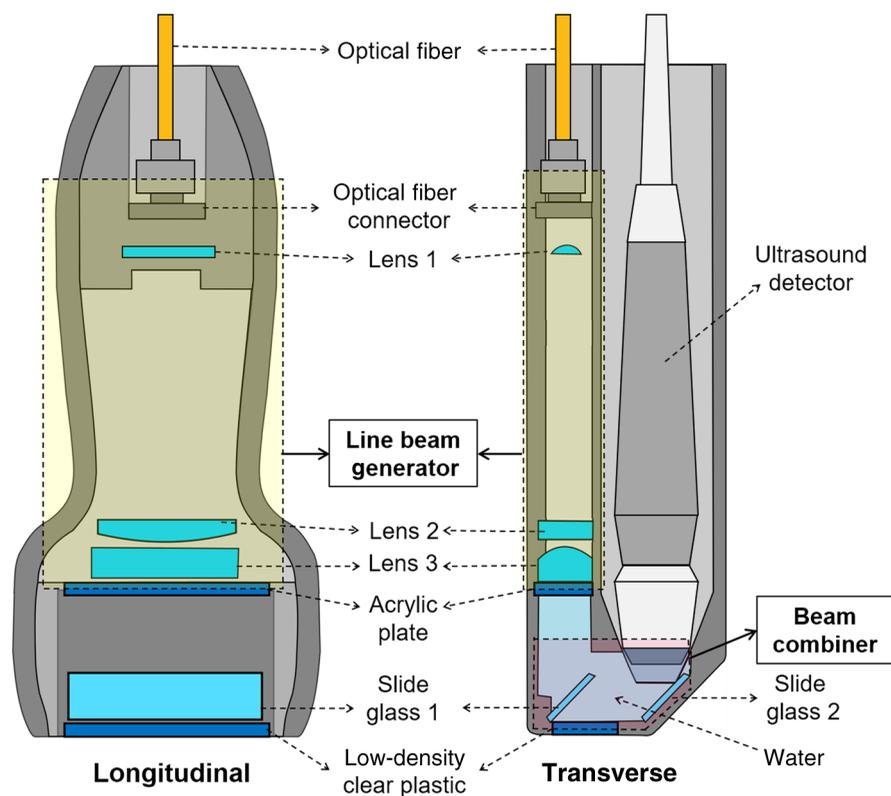
Fig. 2 Schematic of the PAI probe that has the line beam generator and the beam combiner.
