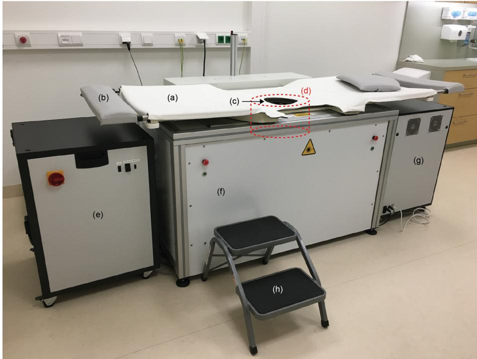
**Fig. 2** The PAM 2 system with (a) the bed on which a woman lies prone, (b) a foot rest, and (c) the breast aperture with (d) a schematic of the shape and position of the imaging tank below the bed, (e) the power supply and cooling unit, (f) laser head (behind the panel), (g) DAQ unit, and (h) step stool.
