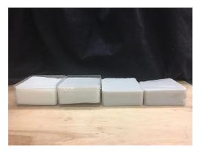
**Fig. 4** Four high contrast solid phantoms for mimicking the chest wall with the size of 10 cm by 10 cm by 4 cm. Their absorption coefficients range from 0.095 to 0.18, and their reduced scattering coefficients range from 5.6 to  $7.1 \text{ cm}^{-1}$ .
