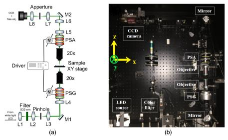
**Fig. 3** Experimental Mueller microscopy set-up in transmission geometry: (a) optical layout: achromatic lenses L1 to L8 (f = 30, 50, 60, 100, 100, 75, 80, and 75, respectively); aluminium mirrors M1 and M2; PSG, polarization state generator; and PSA, polarization state analyser. (b) Side view of the system.
