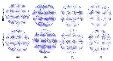
**Fig. 7** The quiver plots of the azimuth of the optical axis obtained with either differential (top row) or Lu–Chipman (bottom row) decomposition and corresponding to the different spatial arrangement of thin sections of corpus callosum: (a) one stripe (10  $\mu$ m), two-layered stack (10  $\mu$ m and 5  $\mu$ m thick stripes) with (b) parallel overlap, (c) overlap at 45 deg, and (d) overlap at 90 deg. The sparse grid with the steps of 20 pixels was used for the visualization.
