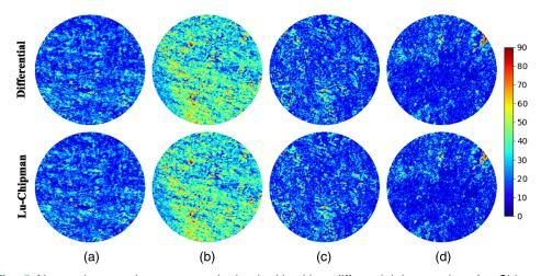
**Fig. 5** Net scalar retardance maps obtained with either differential (top row) or Lu–Chipman (bottom row) decomposition and corresponding to the different spatial arrangement of thin sections of corpus callosum: (a) one stripe (10  $\mu$ m), two-layered stack (10  $\mu$ m and 5  $\mu$ m thick stripes) with (b) parallel overlap, (c) overlap at 45 deg, and (d) overlap at 90 deg.
