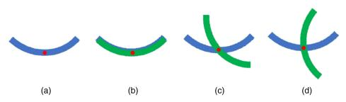
**Fig. 2** Schematics of the spatial arrangement of the histological sections with red spot showing the location of the measurement site: (a) single layer of 10  $\mu$ m nominal thickness, (b) two parallel overlapped layers of 10  $\mu$ m and 5  $\mu$ m of nominal thickness, (c) top layer was rotated by ~45 deg, and (d) top layer was rotated by ~90 deg.
