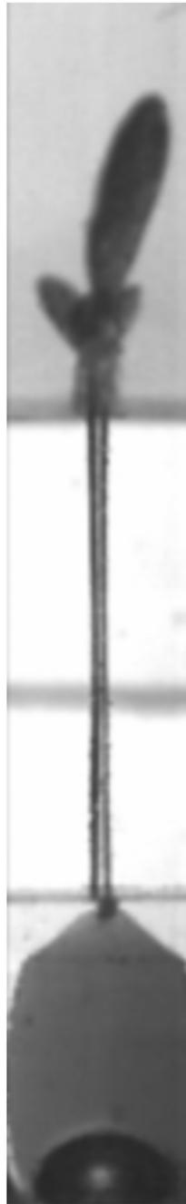
**Fig. 10** Jet penetration into a phantom with 1% agar concentration. The phantom is placed 5 mm away from the chamber. Optical power 1 W and  $\omega_z = 512.3 \mu\text{m}$  ( $z = 34 \text{ mm}$ ). (Video 2, MP4, 1.98 MB [URL: <https://doi.org/10.1117/1.JBO.28.7.075004.s2>]).
