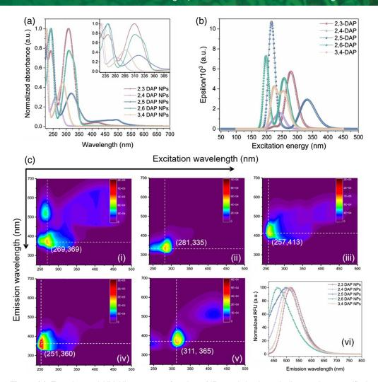
**Fig. 2** (a) Experimental UV–Vis spectra of various NPs and the inset indicates the magnified region between 233 and 390 nm. (b) The predicted spectra of DAP molecules based on DFT calculations. (c) 2D fluorescence map for (i) 2,3 DAP NPs, (ii) 2,4 DAP NPs, (iii) 2,5 DAP NPs, (iv) 2,6 DAP NPs, (v) 3,4 DAP NPs, the emissions centers are identified; and (vi) the normalized emission fluorescent spectra of NPs excited at 360 nm.
