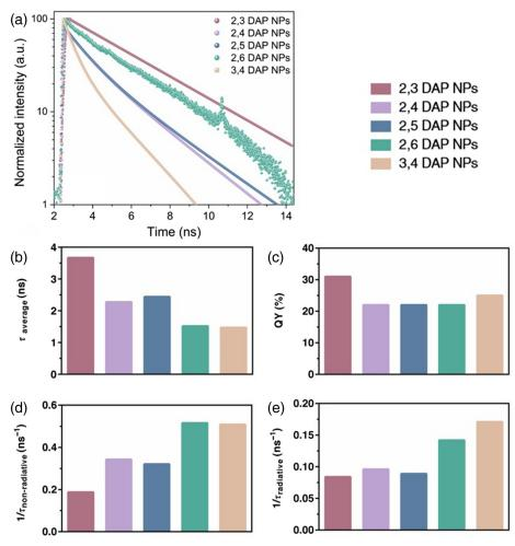
Fig. 5 (a) TRPL spectra of NPs with  $\lambda_{\rm exc}=390$  nm; (b) amplitude weighted average decay lifetime; (c) %quantum yield (QY) values for the five different DAP nanoparticles synthesized herein; (d) non-radiative decay rate; and (e) radiative decay rate.
