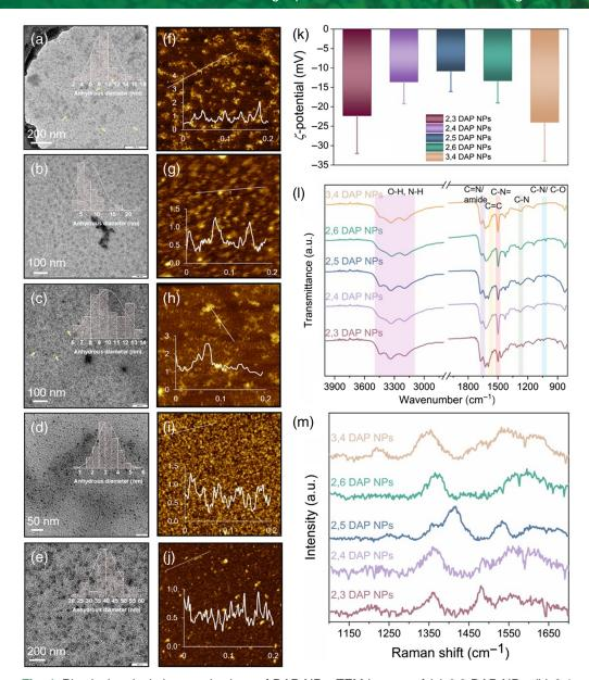
**Fig. 1** Physiochemical characterizations of DAP NPs: TEM images of (a) 2,3 DAP NPs, (b) 2,4 DAP NPs, (c) 2,5 DAP NPs, (d) 2,6 DAP NPs, (e) 3,4 DAP NPs; AFM images and the height distribution for (f) 2,3 DAP NPs, (g) 2,4 DAP NPs, (h) 2,5 DAP NPs, (i) 2,6 DAP NPs, (j) 3,4 DAP NPs; (k) electrophoretic zeta potential; (l) FTIR; and (m) Raman spectra of NPs.
