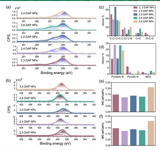
**Fig. 3** Deconvoluted (a) C1s region and (b) N1s region; (c) the comparison of various C-containing functional groups; (d) N-containing functional groups; and (e) the O/C and (f) N/C atomic percent distribution for different NPs.
