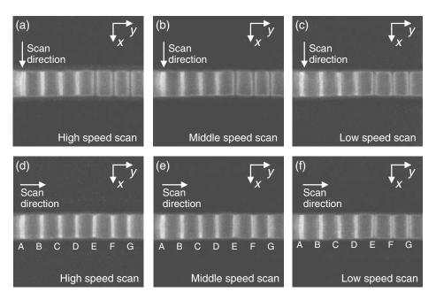
**Fig. 9** VC images with different scan speeds and directions. (a)–(c) Scan parallel to NWs with high-, middle-, and low-speed scans, respectively. (d)–(f) Scan across NWs with high-, middle-, and low-speed scans, respectively. Capital letters A to G indicate NWs whose profiles are shown in Fig. 10.
