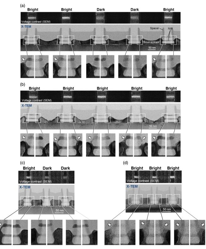
**Fig. 8** Comparison between SEM VC images and cross-sectional TEM images of the NWs. (a) 70-nmlong NWs at wafer edge, (b) 70-nm-long NWs at wafer center, (c) 28-nm-long NWs at wafer edge, and (d) 28-nm-long NWs at wafer center. White arrows in enlarged TEM images are indicating that NW and SD are connected through a narrow bridge.
