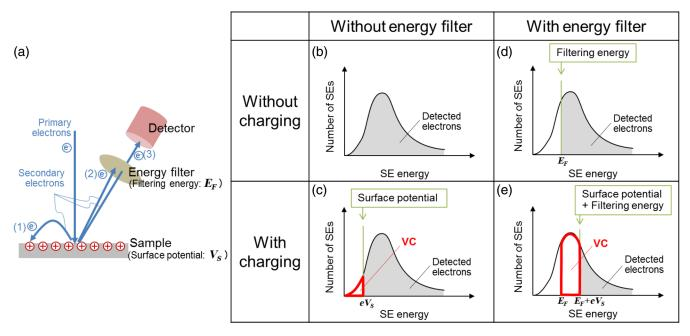
**Fig. 3** (a) A schematic illustration of SEM signal detection from positively charged sample with an energy filter. SE spectrum (a) without charging and without an energy filter, (b) with charging and without an energy filter, (d) without charging and with an energy filter, and (e) with charging and with an energy filter. Shared area corresponds to the detectable electrons. Area surrounded by bold lines corresponds to VC. VC is enhanced by energy filtering.
