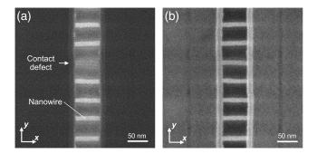
**Fig. 6** Typical SEM images of 70-nm-long NWs. (a) An SEM image acquired with energy filtering of SEs. (b) A SEM image acquired without energy filtering. Both images were taken with 800-V accelerating voltage, 8-pA probe current, and middle-speed scan along x axis. They are the same NWs. VC is clearly observed by energy filtering.
