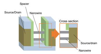
Fig. 2 Schematic configuration of NW FET and its cross-section parallel to the NW.
