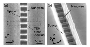
Fig. 4 An example of (a) top-view SEM image of the NW sample and (b) a tilted SEM image.
