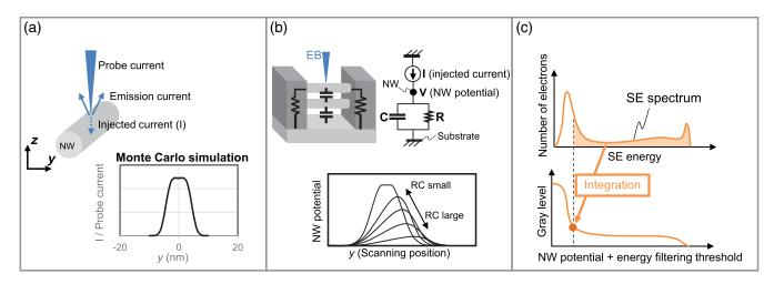
Fig. 5 Overview of the proposed model to calculate VC. (a) Injected current calculation step, (b) NW potential calculation step, and (c) gray-level estimation step.
