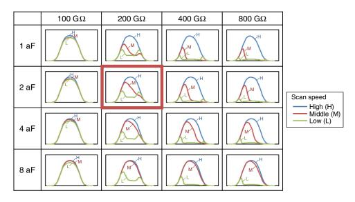
**Fig. 11** VC profiles calculated by the proposed VC model. About 16 combinations of resistance ( $R = 100, 200, 400, and 800 \text{ }\Omega\Omega$ ) and capacitance (C = 1, 2, 4, and 8 aF) were used as input parameters of the model. Among these series of VC profiles, the result with  $R = 200 \text{ }\Omega\Omega$  and C = 2 aF is most similar to the experimental result.
