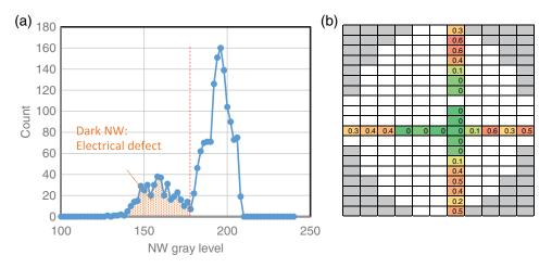
**Fig. 7** (a) Gray-level histogram of 1680 70-nm-long NWs. Gray level was extracted from the VC images taken with 800-V accelerating voltage, 8-pA probe current, and middle-speed scan along x axis (parallel to NWs). The dashed line is a criterion between dark NWs and bright NWs. The dark NWs should correspond to the electrical defects. (b) Intrawafer map of the ratio of defect NWs. Electrical defects are more frequent at wafer edge.
