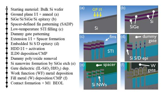
Fig. 1 Process flow of Si NW FETs fabrication.
