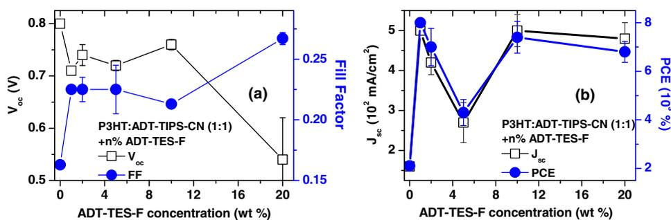
**Fig. 8** (a)  $V_{oc}$  (left axis) and FF (right axis) and (b)  $J_{sc}$  (left axis) and PCE (right axis) obtained in ternary P3HT:ADT-TES-F:ADT-TIPS-CN (1:  $x$ : 1) blends as a function of ADT-TES-F concentration in the 0 to 20 wt% range ( $x = 0$  to 0.5). Each value represents an average over four devices, and error bars reflect spread in values.
