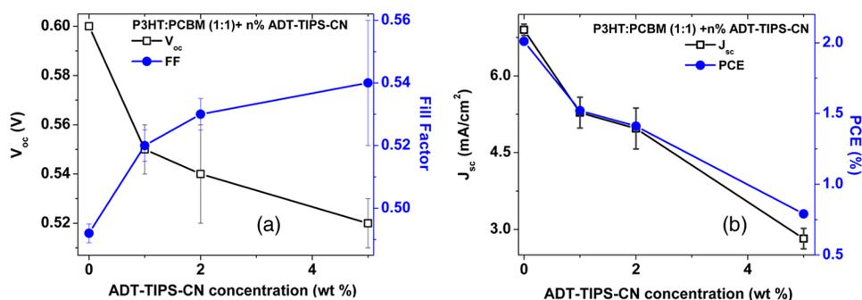
**Fig. 7** (a)  $V_{oc}$  (left axis) and FF (right axis) and (b)  $J_{sc}$  (left axis) and PCE (right axis) obtained in ternary P3HT:PCBM:ADT-TIPS-CN (1:1: $x$ ) blends as a function of ADT-TIPS-CN concentration in the 0 to 5 wt% range ( $x = 0$  to 0.1). Each value represents an average over four devices, and error bars reflect spread in values.
