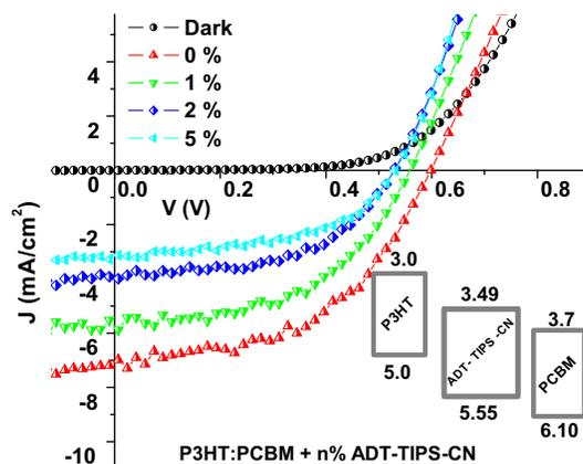
**Fig. 6** J-V curves obtained in ternary P3HT:PCBM:ADT-TIPS-CN (1:1:x) solar cells at various concentrations of ADT-TIPS-CN in the 0 to 5 wt% range ( $x = 0$  to 0.1). Dark current in the binary blend ( $x = 0$ ) is also included. Inset shows HOMO and LUMO energies of molecules.
