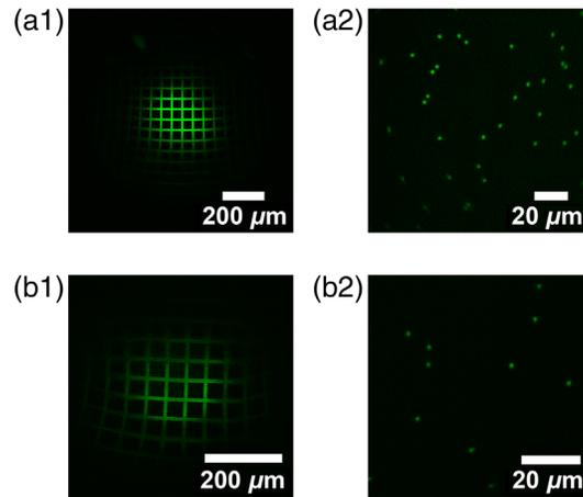
**Fig. 2** Two-photon optical characterizations of the GRINtrode imaging systems at 920 nm. 50- $\mu\text{m}$  grid slide calibration target used for FOV measurements using the GRIN lens imaging system A (a1) and imaging system B (b1). 0.5- $\mu\text{m}$  fluorescent bead slide sample used for lateral and axial FWHM measurements using the GRIN lens imaging system A (a2) and imaging system B (b2).
