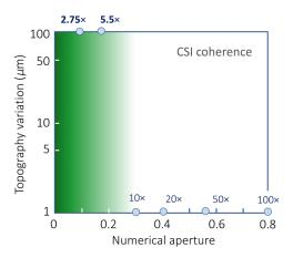
**Fig. 13** Limits to applicability of the EFO model for CSI for coherence profiles using common light sources. The white light approximation is limited to low NA values characteristic of objective magnifications below 10×.
