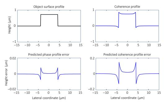
**Fig. 9** Simulated results using the EFO model for an 8- $\mu$ m wide rectangular surface feature with a height of 0.75  $\mu$ m. The mean wavelength is 0.57  $\mu$ m, the FWHM bandwidth is 0.12  $\mu$ m, and the NA is 0.15. Note the 10× difference in height scale for the predicted errors for the coherence and phase profiles.
