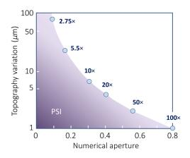
**Fig. 11** Limits to the allowable surface height variation for the use of the EFO model for a fixedfocus (nonscanning) system based on the DOF. The graph includes representative magnifications for common interference objectives.
