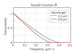
Fig. 6 The imaging TF calculated from Eq. (16) for wavelengths 0.5 and 0.6  $\mu$ m.
