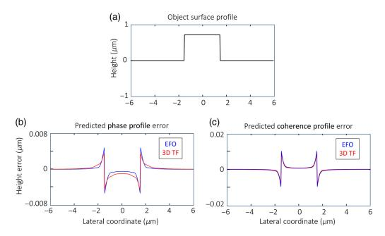
**Fig. 16** (a) Simulations for the EFO and 3D TF models NA = 0.55 (50× objective), for a rectangular profile similar to that shown in Fig. 9, with a width of 3  $\mu$ m and a height of 0.75  $\mu$ m. The mean wavelength is 0.57  $\mu$ m and the bandwidth is 0.14  $\mu$ m. The predicted measurement errors for (b) the phase profile and (b) the coherence profile.
