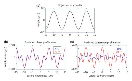
**Fig. 15** (a) Simulations for the EFO and 3D TF models at NA = 0.55 (50× objective) for a sinusoidal profile with an amplitude of 0.15  $\mu$ m. The mean wavelength is 0.57  $\mu$ m and the FWHM bandwidth is 0.08  $\mu$ m. The predicted measurement errors for (b) the phase profile and (c) the coherence profile.
