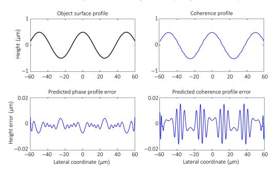
**Fig. 8** Simulated measurement results using the EFO model for the profile of Fig. 1. The sinusoidal period is 50  $\mu$ m, and the peak-valley height range is 1  $\mu$ m. The mean wavelength is 0.5  $\mu$ m, the FWHM bandwidth is 0.1  $\mu$ m, and the NA is 0.1.
