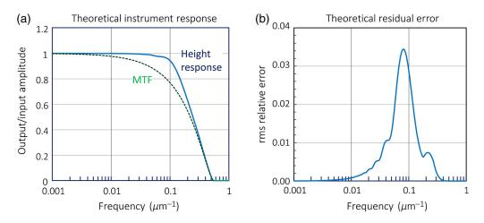
**Fig. 10** EFO modeling analysis of instrument response as a function of surface spatial frequency for phase profiles, for a constant maximum surface slope equal to 50% of the geometrical NA limit. (a) The results in comparison with the optical imaging MTF and (b) the rms error in the measured profile. The mean wavelength is 0.57  $\mu$ m and the NA is 0.15.
