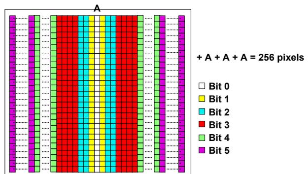
Fig. 16. TDI scheme makes the DPG much less to contaminations.
