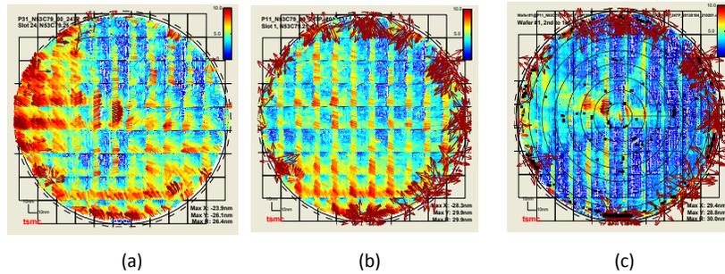
Fig. 2. (a) and (b) are overlay maps after the 1<sup>st</sup> and the 10<sup>th</sup> pass through the contaminating tool. Figure 2(c) is the contamination map from an optical microscope.
