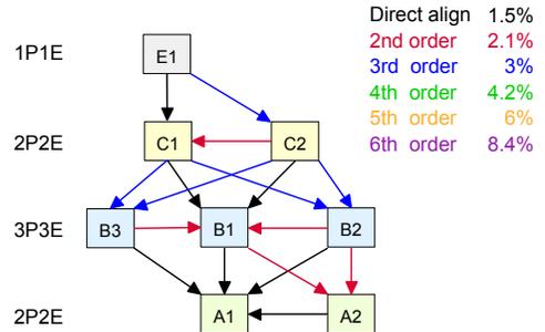
Fig. 6. Overlaying a 1P1E layer on multiply patterned layers cannot eliminate high-order alignments.
