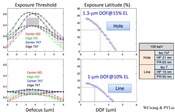
Resist scattering and 10-nm blur by acid diffusion are included.
