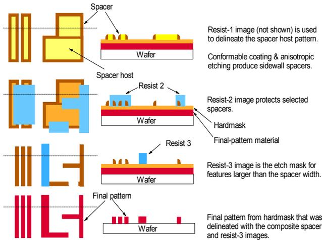
Fig. 8. The spacer technique to double resolution.
