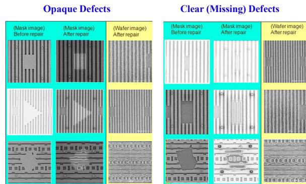
Fig. 13. Sample EUV opaque and clear defects, before and after repair.
