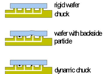
Fig. 3. (top to bottom) rigid wafer back referenced chuck; Sane chuck distorting a contaminating wafer; Dynamic front-referenced chuck.
