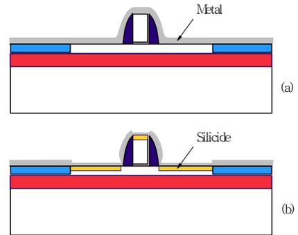
Fig. 7 Self-aligned silicide process
