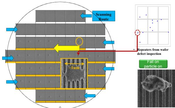
Fig. 14. A micrometer-size particle deposited on the EUV mask during scan-and-repeat exposure.
