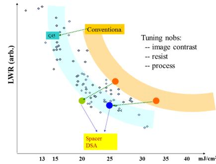
Fig. 11. Tradeoff between LWR and resist sensitivity
