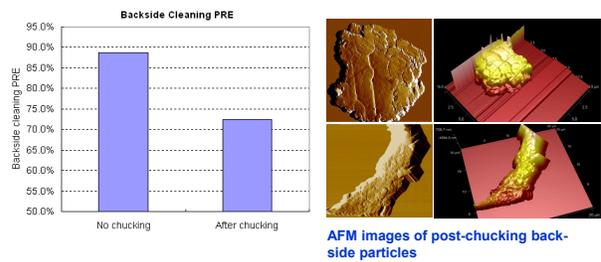
Fig. 15. Particle removal efficiency of chucked and unchucked masks with backside particle.
