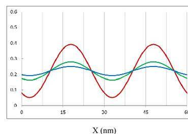
Fig. 10. Simulated EUV image intensity of 30-nm pitch gratings at resist blurs=0, 7, and 9 nm. The pitch of the image is 30 nm.
