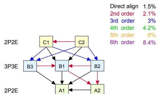
Fig. 5. Overlay tree of 2P2E aligned to 3P3E on 2P2E. Indirect alignments up to the 3<sup>rd</sup> order are present.
