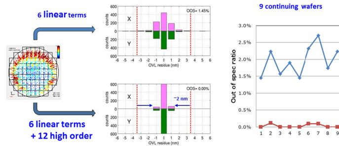
Fig. 4. Overlay accuracies with and without high-order corrections.
