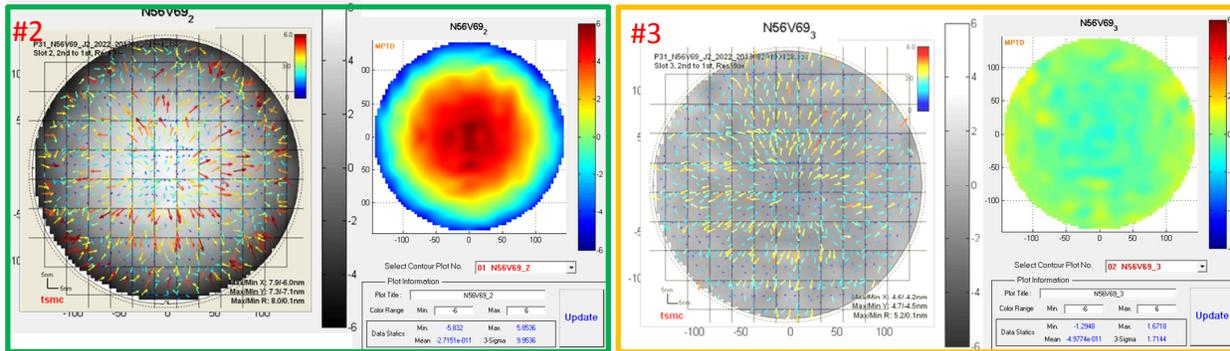
Fig. 1. Wafer #2 has a TiN layer which was skipped for wafer #3. The warpage was measured with a Zygo interferometer showing a range of 11.6  $\mu\text{m}$  and 2.96  $\mu\text{m}$  respectively. The overlay errors are 8 and 5.2 nm.
