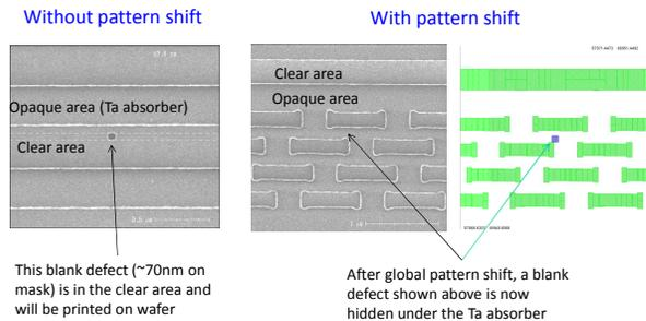
Fig. 12. Global mask pattern shift to mitigate EUV mask blank defects.
