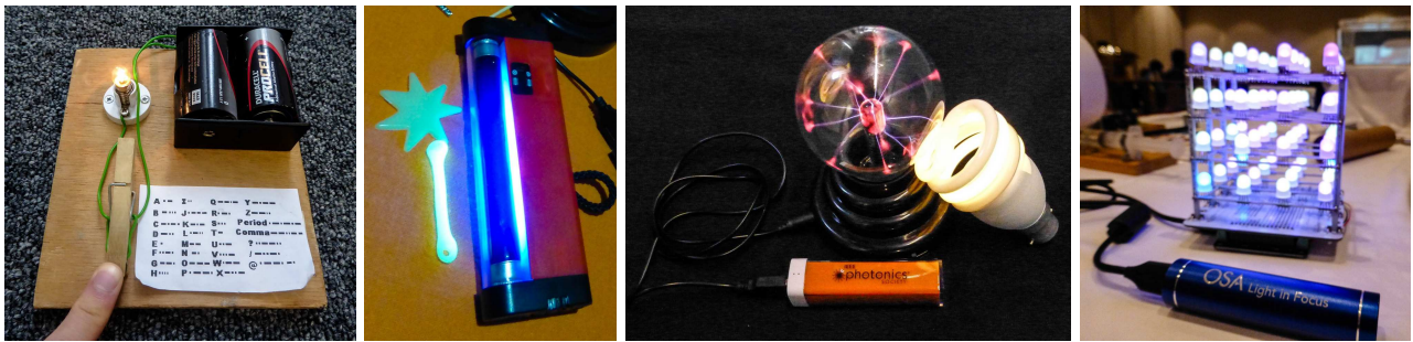
Figure 2: (Left to right) Battery operated kits: Morse code circuit, and ultraviolet lamp; and powerbank operated kits: plasma globe and fluorescence bulb, and LED matrix.
