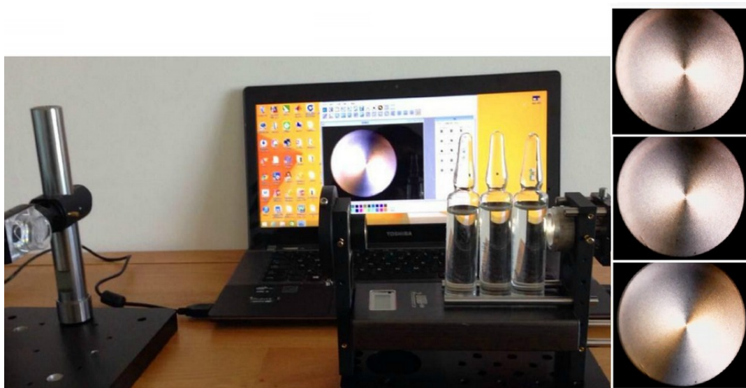
Fig. 7 A mounted lens and glasses with obvious and large strain distribution.
