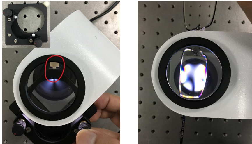
Fig. 6 A mounted lens and glasses with obvious and large strain distribution.
