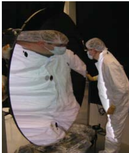
Fig 4. Coated primary mirror in SiC
