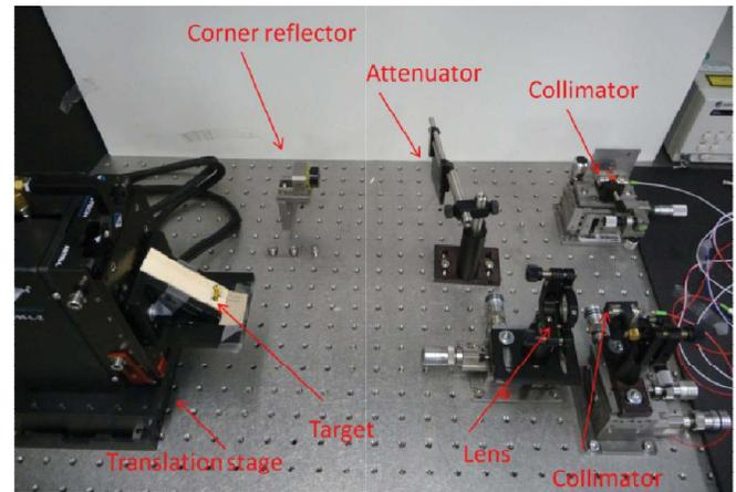
Fig. 5. Photo of the SAL laboratory set-up
