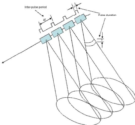
Fig. 1. Illustration of a SAR image acquisition system
