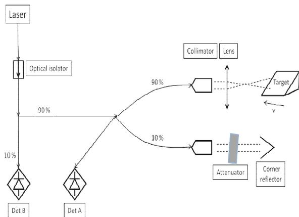
Fig. 4. Schematic of the SAL laboratory set-up
