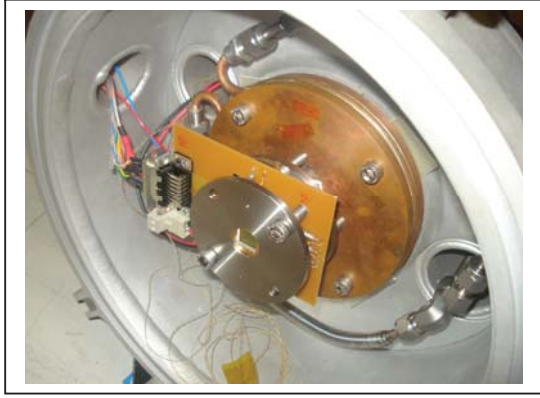
Figure 5. Vacuum chamber with Cactus mounted inside before vacuum pumping
