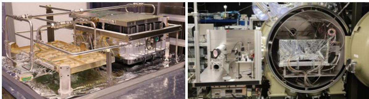
Figure 7: Left : Laser in preparation for thermal vacuum testing; Right : test facility with integrated laser and external test setup for online laser performance measurement
