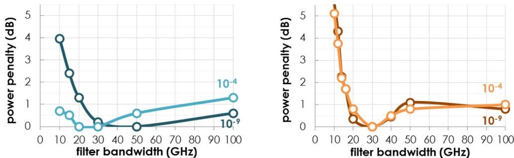
Figure 6. Influence of optical filter bandwidth on detection sensitivity for 10 Gbps NRZ OOK (left) and NRZ DPSK (right)
