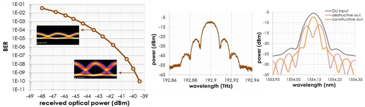
Figure 5. BER for a 10 Gbps NRZ DPSK signal (left), eye diagrams at  $10^{-4}$  and  $10^{-9}$  (inset), optical spectrum at Tx output (center) and optical spectra at each output of the delay line interferometer (right).
