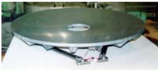
SiC Brazing technic have been validated for the manufacturing of the Ø 1.35 meter mirror demonstrator (FIRST breadboard: see [4];[5] & [6] )
