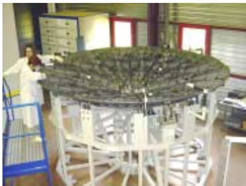
Mirror assembly prior brazing phase
