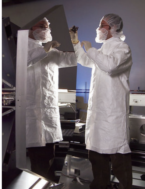
Figure 12: A JWST hexagonal segment is shown during optical finishing at L-3 Tinsley. An average clear-aperture allowance around the edge of 5 mm was achieved while polishing the lightweight segment from the start in hexagonal form. (NASA Photograph...)
