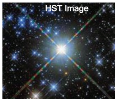
Figure 2 HST image of a star showing the diffraction spikes that mask exoplanets at 4 position angles. The halo around the star is produced in the telescope/instrument system by narrow angle scattered light. The Airy diffraction pattern for HST is about 100 milliarc seconds which is too large to observe terrestrial exoplanets 1 astronomical unit from the parent star.
