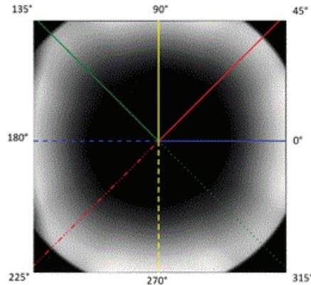
Figure 9 Flat filed image with lines from the centre to the edges at the angles 0°- 180° (blue lines); 45°- 225° (red lines); 90°-270° (yellow lines); 135°-315° (green lines).
