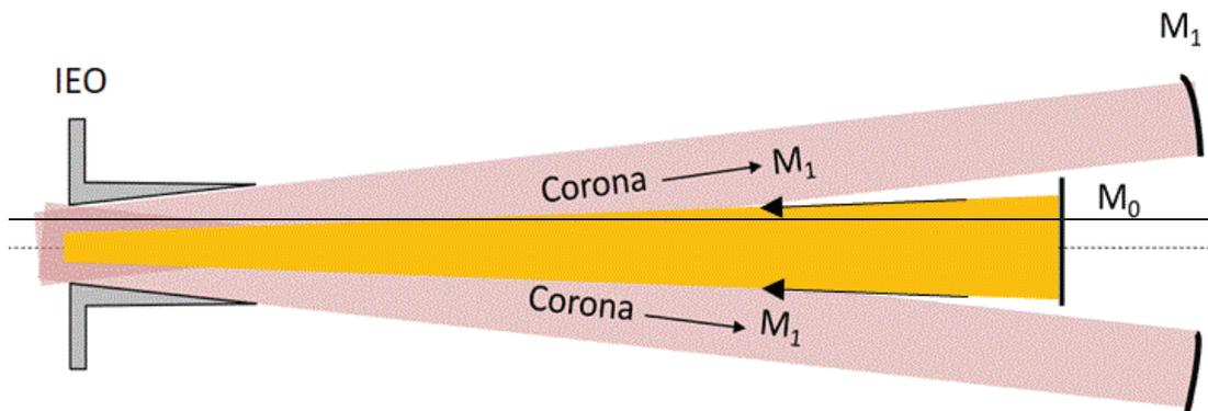
Figure 1 Schematic view of the Metis occultation. The light from the solar disk is back rejected by  $M_0$  (yellow). The light of the corona passes inside the coronagraph.
