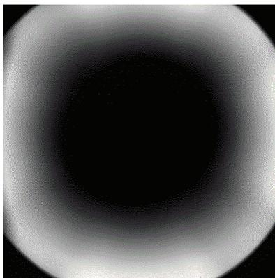
Figure 5. Image of the flat field panel after the subtraction of the dark.
