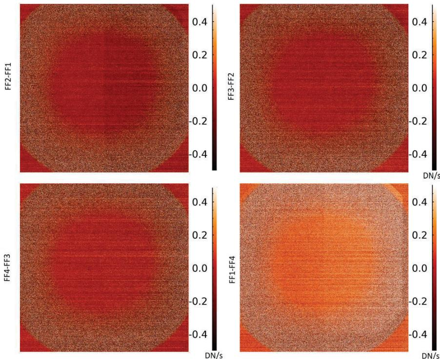
Figure 6. Flat field difference of 4 images acquired with  $t_{exp}=100$ s, in DN/s, i.e. divided by the integration time.
