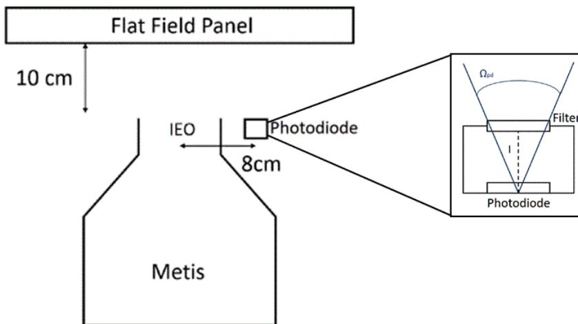
Figure 4 Diagram of the top and sectional view of the flat field panel, of the photodiode and of Metis with relative distances and with a zoom of the photodiode and its filter.
