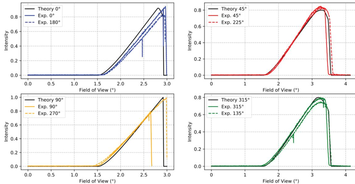
Figure 10. Trends of the flat field curve with varying angles: 0°- 180°, 45°- 225°,90°-270° and 135°-315°, normalized at the maximum value measured in the 270° direction. The black lines, denoted with “Theory”, are the ones calculated with the Zemax raytracing code, while the coloured “Exp” the measured ones.
