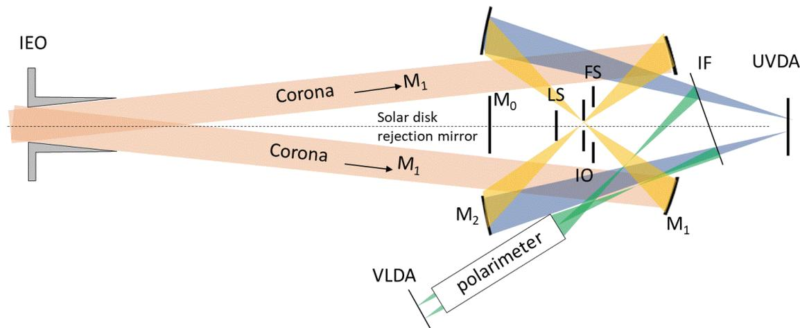
Figure 2 Schematic view of Metis coronagraph for both the UV and Visible Light channel.
