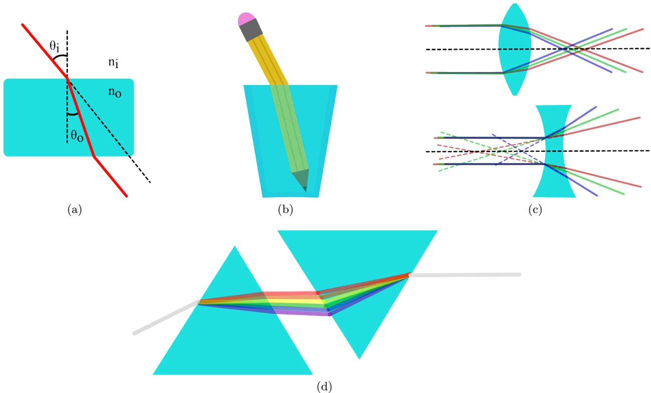
Figure 18. Snell law experiments (a) A parallel faces film, (b) Seen the refraction of a pencil in a glass of water, (c) Rays of different wavelength through convergent and divergent lenses. (d) Scattering light through two prisms.
