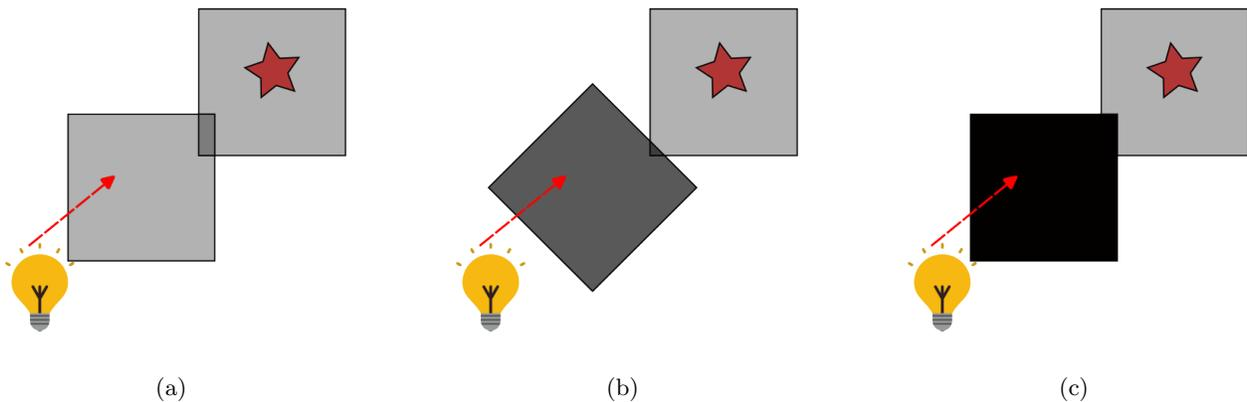
Figure 8. Light propagation through two polaroids. (a) parallel direction of polarization, (b) rotated polarization angle and (c) orthogonal direction of polarization.
