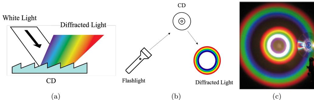
Figure 2. Diffraction through a CD. (a) Conceptual sketch of the working principle of a diffraction grating, adapted from Edmund Optics.<sup>5</sup> (b) Conceptual sketch of the experimental procedure. (c) Experimental result, figure taken from Ivanov *et al.*<sup>6</sup>
