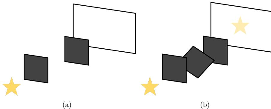
Figure 10. Experimental demonstration of the vectorial behavior of light. (a) when two perpendicular-oriented linear polarizers there is no transmission of light, but (b) when another polarizer at oriented at  $45^\circ$ , a diagonal polarization state is generated and there is transmission.
