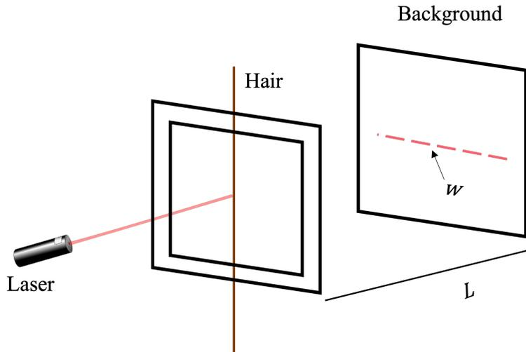
Figure 3. Conceptual sketch of a double slit experiment carried out with a human hair.  $L$  is the distance between the hair and the solid background.  $w$  is the distance between luminous points.
