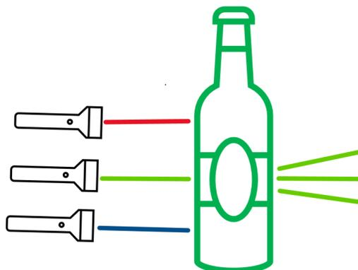
Figure 6. Behavior of red, green and blue light through a green bottle (color filter).
