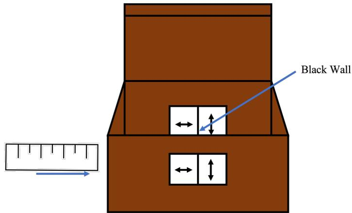
Figure 9. Conceptual sketch of the magic box experiment. The black wall is generated because of the perpendicularity of the two polarizers of the box.
