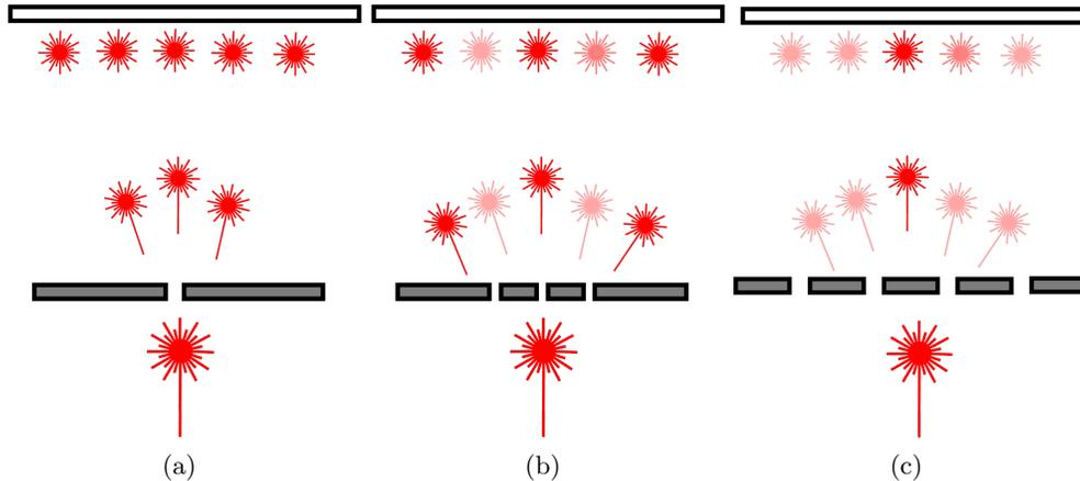
Figure 1. Conceptual sketch of a diffraction grating experiment. The dimmer points represents subsidiaries maximums, while the luminous points represents principal maximums. (a)-(c) displays the relation between the dimmer points and the number of slits.
