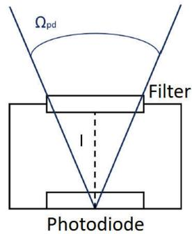
Figure 4 Scheme of the photodiode and filter.
