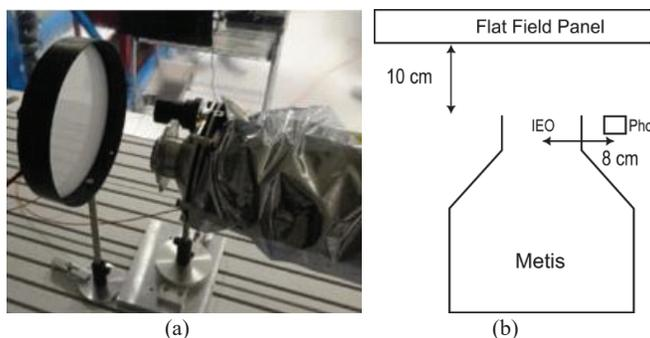
Figure 3 (a) Optical layout of Metis in the laboratory calibration test set-up. (b) Diagram of the top view of the flat field panel, of the photodiode and of Metis with relative distances.
