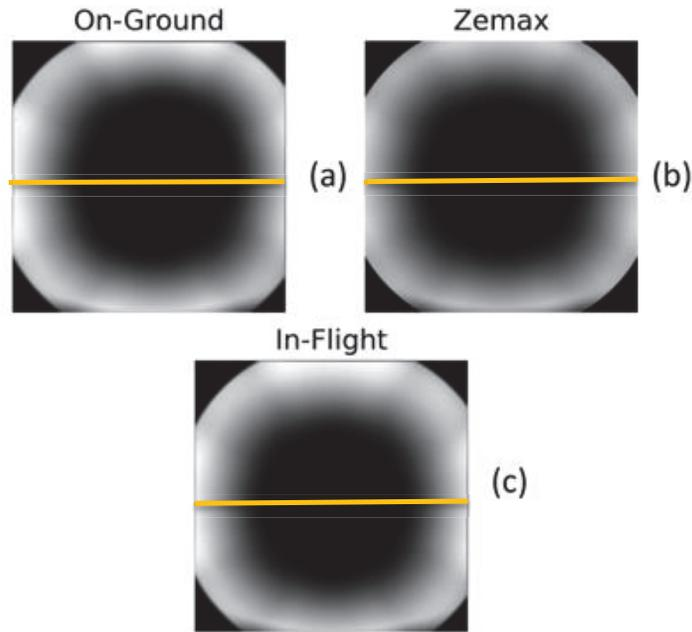
Figure 5 Images of the vignetting function acquired on-ground (a), simulated by Zemax (b), adjusted in-flight (c). The orange lines are the position of the plot of the vignetting.
