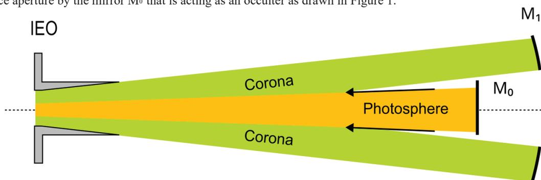
Figure 1 Schematic view of the Metis occultation concept. The light from the solar disk (dark yellow) is back rejected by the mirror  $M_0$ . The light of the corona (green) passes and enters inside the coronagraph.
