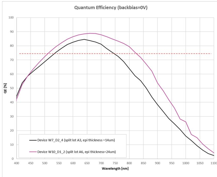
Figure 7: Spectral response measurement of an ELFIS2 sensor with an epi thickness of 12, respectively 22  $\mu\text{m}$ .
