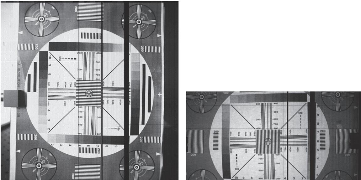
Figure 6: Image of an EIA-1956 test chart in full resolution (Left) and an image with a vertical ROI between rows 512 and 1536. (Right)
