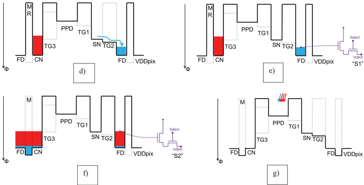
Figure 2: a) Simplified floor plan of the ELFIS pixel with the Contour (red dashed line) for the potential profile discussions - b) to g) potential diagrams during the different phases of the charge accumulation and read-out cycle.
