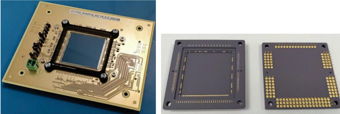
Figure 5: Left: Present CoB assembly of the first ELFIS2 devices - Right: package for the future flight devices
