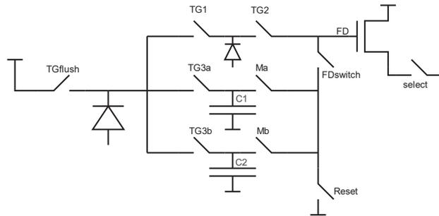
Figure 1: Schematic representation of the new ELFIS2 Pixel. FD isolation is highlighted.
