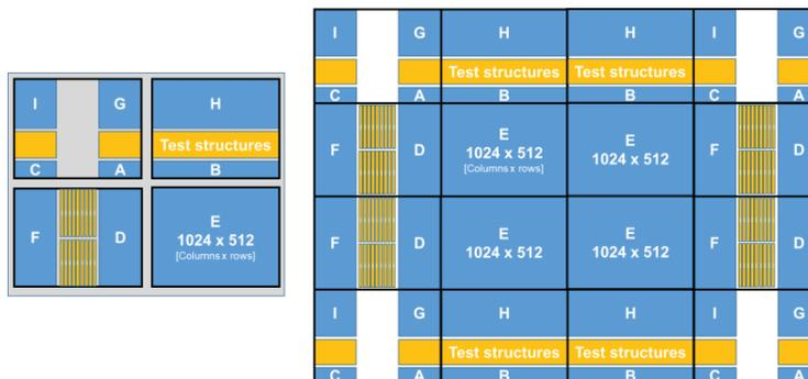
Figure 3: Left: Reticle design with the 4 stitch blocks- Right: stitched configuration for a 2k\*1k design.
