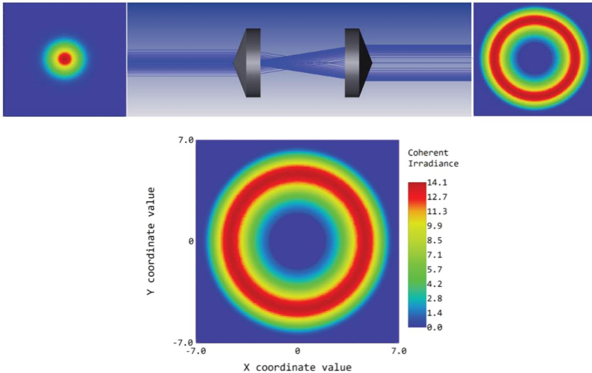
Figure 3. Light distribution of the annulus generated by the axicon pair from a collimated gaussian beam.
