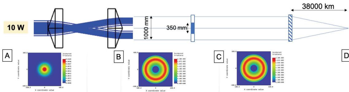
Figure 6. Physical optics propagation of the annulus exiting the axicon pair to a distance of 38000 km.
