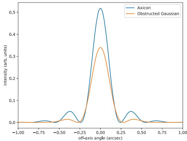
Figure 8. Comparison of the Point Spread Functions (corresponding to location D in Figure 6 and location C in Figure 7) of a beam after being shaped by an axicon pair and a gaussian beam obstructed by the secondary mirror. PSFs computed using AOTools.<sup>8</sup>
