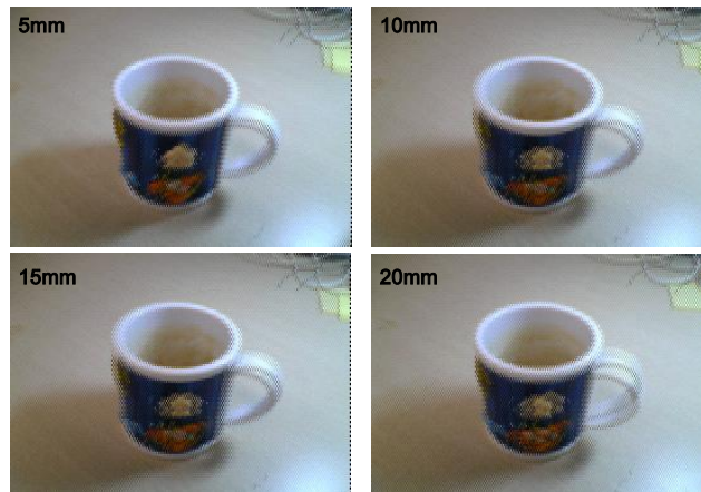
Fig. 1. Combined Left and Right Images for Different Base distances When the distance between HPh camera and object is 21cm
