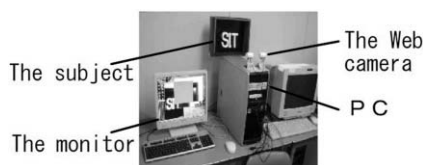
Fig. 5 The kinoform creation and photography environment.
