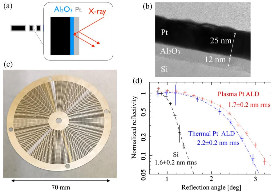
**Fig. 9** (a, c) Concept and photo of Pt-coated MEMS x-ray optics, (b) a transmission electron microscope image of a sidewall, and (d) x-ray reflectivity curves at  $AlK_{\alpha}$  1.49 keV of the sidewalls. The photo and electron microscope image are for the plasma Pt ALD sample, while the reflectivity curves are for both the thermal and plasma Pt ALD samples. Numbers indicate microroughness estimated from the reflectivity curves.
