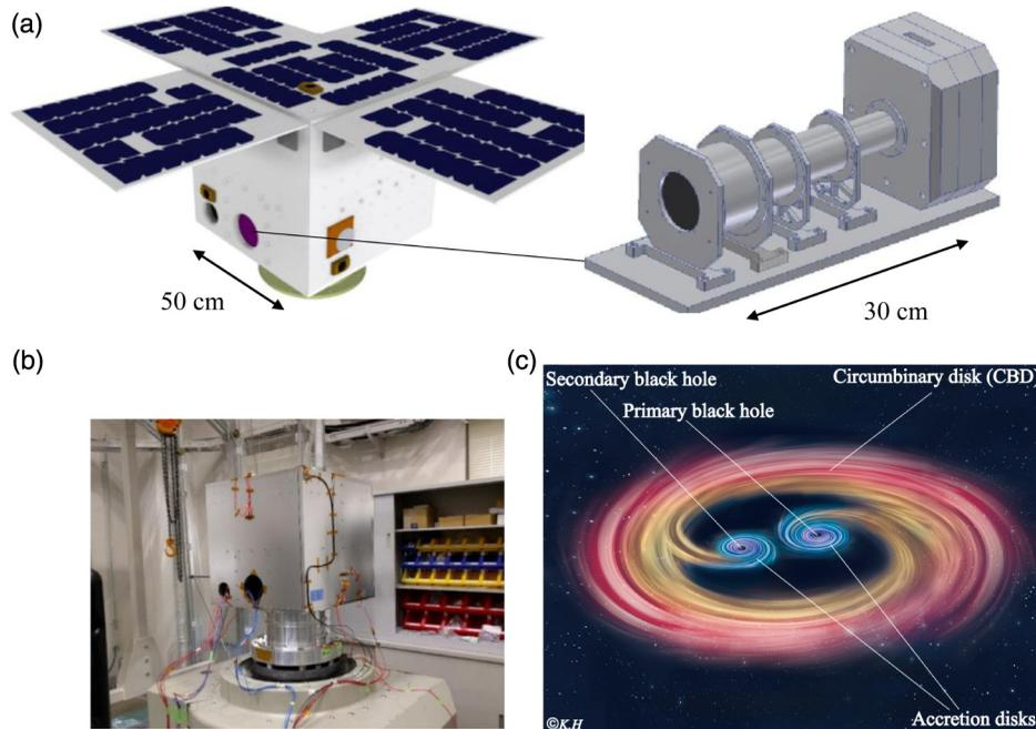
**Fig. 2** Overview of the ORBIS mission: (a) three-dimensional cad drawings of the spacecraft and the payload, (b) a photo of a structure and thermal model,<sup>15</sup> and (c) artistic impression of a BBH.<sup>17</sup>
