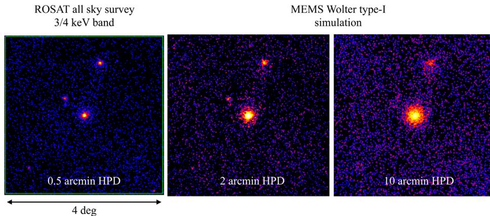
**Fig. 10** MEMS Wolter type-I simulations compared to an original ROSAT all-sky survey 3/4 keV band image near the Galactic center ( $ra, dec = (266.404996, 28.936172)$  in J2000.<sup>38</sup> The parameters for the MEMS Wolter type-I optic are summarized in Table 5. An x-ray energy of 0.6 keV is assumed. The exposure time of the original ROSAT image is  $\sim 290$  s, while the assumed exposure time for each MEMS Wolter type-I simulation image is set at  $\sim 8$  ks.
