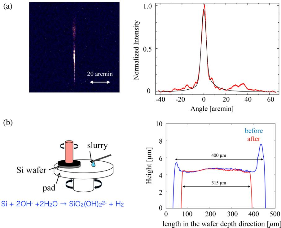
**Fig. 8** (a) X-ray response of a single mirror after DRIE and annealing at  $\text{AlK}_\alpha$  1.49 keV and its projected profile fitted with Gaussian and Lorentzian models. (b) Concept of chemical mechanical polishing and an example of sidewall profiles of a sample DRIE-fabricated optic before and after polishing.
