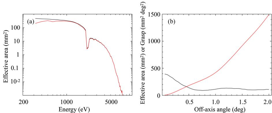
**Fig. 7** (a) Effective area of the MEMS Wolter type-I optic estimated from the raytracing simulations. Black and red curves represent an effective area without and with a detector quantum efficiency and an optical blocking filter. (b) Grasp of the MEMS Wolter type-I optic as a function of off-axis angle. Black and red curves are an effective area and a grasp. The detector and optical blocking filter efficiency is not included.
