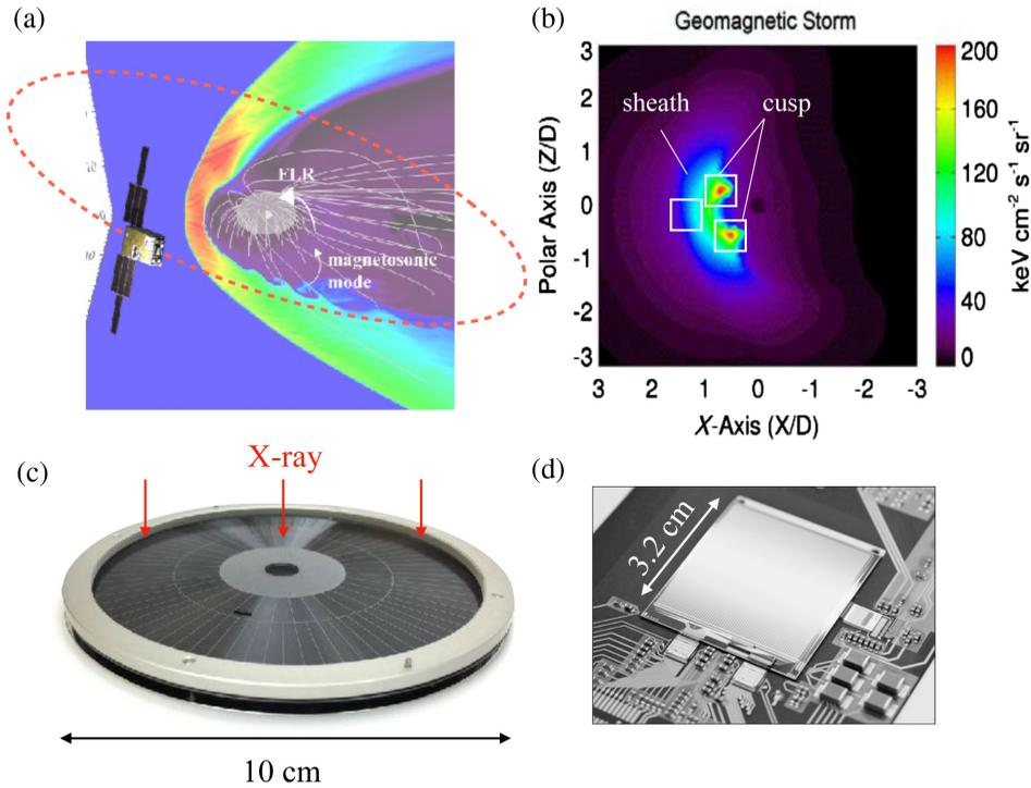
**Fig. 3** Overview of the GEO-X mission: (a) a concept of the spacecraft orbiting around the Earth’s magnetosphere,<sup>30</sup> (b) an MHD-based model for the solar wind charge exchange emission as observed from  $50 R_{\text{Earth}}$ ,<sup>29</sup> (c) an MEMS Wolter type-I optic, and (d) a DepFET detector.<sup>31</sup> Each solid square in the MHD simulation indicates a FOV of the payload.
