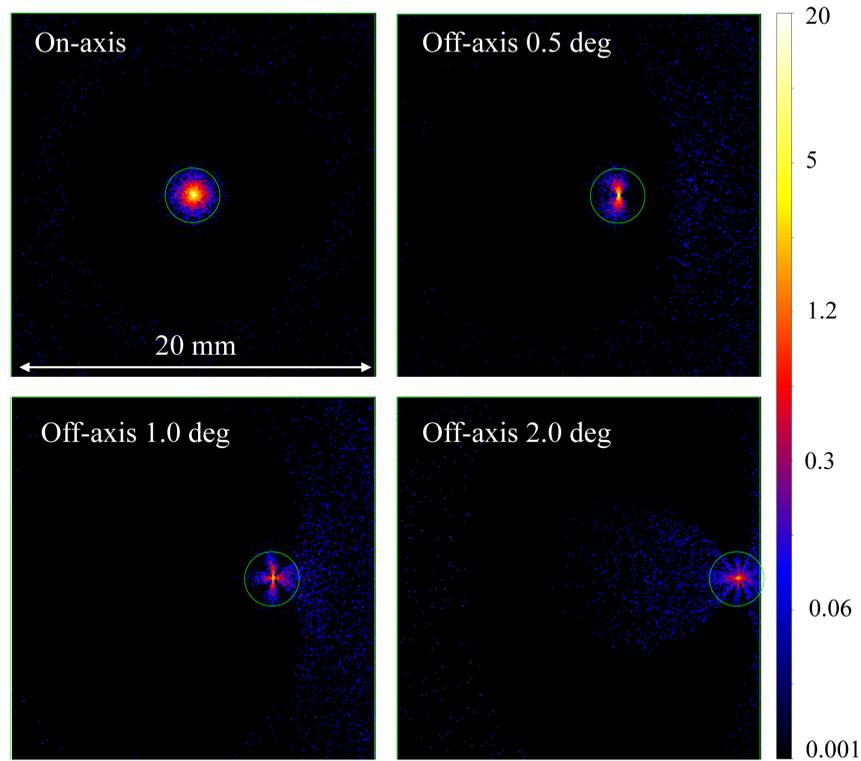
**Fig. 6** Raytracing results for the MEMS Wolter type-I optic assuming optics parameters in Table 5 at 0.6 keV. Different incident angles are used. A color scale is in arbitrary unit. A solid circle corresponds to an area with a radius of 1.5 mm used for the effective area and grasp calculations.
