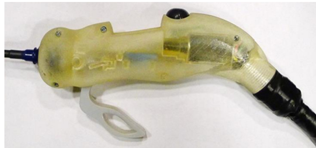
Fig. 4 The handle of the articulating tip confocal microlaparoscope probe. The design incorporates an articulation lock that allows setting and maintaining a specific angle at the distal tip. A multipurpose button on top of the probe allows the operator to deliver contrast agent and grab static images.
