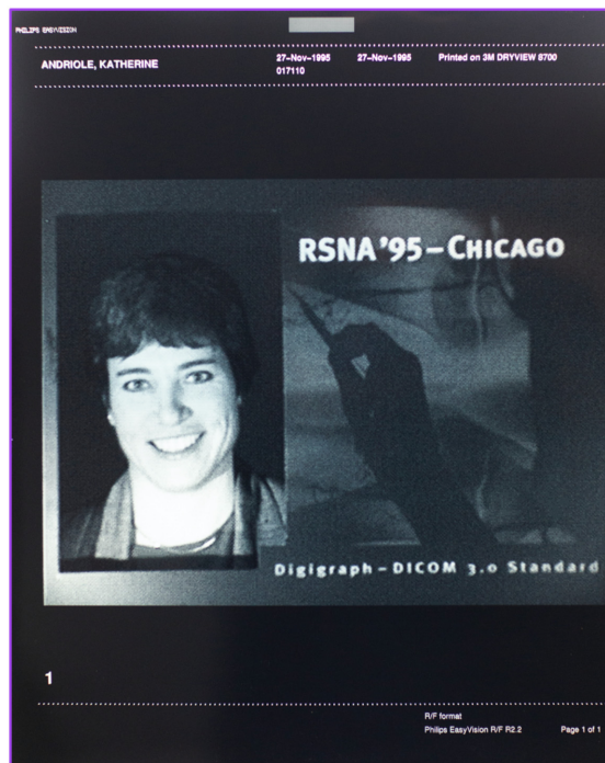
Fig. 2 DICOM demonstration at RSNA InfoRAD. Image acquired on vendor X device (upper left corner) and displayed/printed on vendor Y device (upper right corner) demonstrating the DICOM standard file format and communications protocol. Personal photo from 1995 RSNA Conference courtesy K.P. Andriole.
