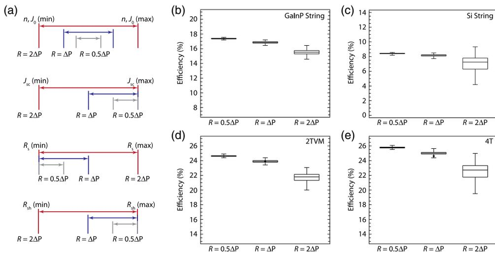
**Fig. 4** Results of 3:1 minimodule simulations. (a) Schematic of how the parameter ranges,  $P$ , were varied for the simulations. Efficiencies are plotted for all three  $P$  ranges for (b) the GaInP<sub>2</sub> string, (c) the Si string, (d) the 2TVM tandem, and (e) the 4T tandem. The circular markers in (d) and (e) represent the experimentally-measured module values.
