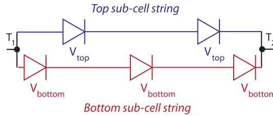
**Fig. 1** Generalized schematic of a two-terminal VM tandem module.
