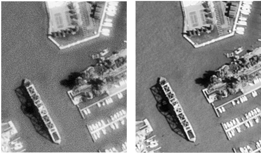
Fig. 2 Simulations from imaging chain models allow us to see image quality differences from two camera designs that have the same top-level requirements but subtle differences in the component designs. The image on the left was created from a design option that explored lowering the manufacturing cost, but this process increased optical aberrations and used a sensor with lower sensitivity, resulting in a noticeable image quality degradation in the image simulations.
