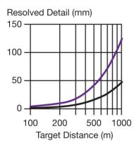
This graph plots resolved detail (in mm) at the target distance L (in m) on a horizontal path for medium air turbulence (colored curve) and weak turbulence (black curve). As expected, increased turbulence reduces the amount of detail that can be resolved at any distance.
