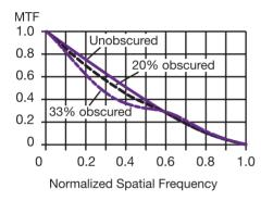
MTF is plotted here for three values of obscuration:  $\varepsilon=0$ , (unobscured),  $\varepsilon=0.20$  (typical of a Newtonian scope), and  $\varepsilon=0.33$  (typical of a Schmidtor a Maksutov–Cassegrain scope). The normalized spatial frequency is  $\nu_n=\nu\lambda/D_{EP}$ . Here  $\nu$  and  $\nu_n$  are in cycles/mm.
