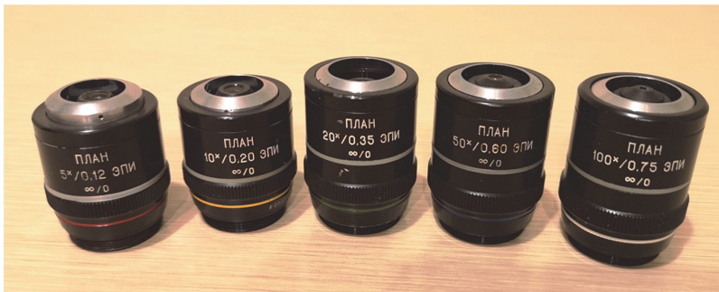
Figure 1.272 Set of metallographic LCF plan achromatic objectives for an infinite length of the tube.
